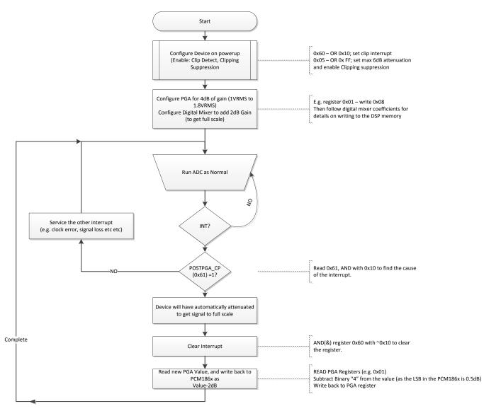
Figure 5. Workflow to Use Auto Gain Suppression With a -2 dBFS Input Signal
