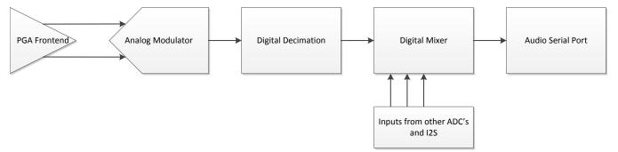
Figure 1. ADC Signal Chain Architecture of PCM186x
