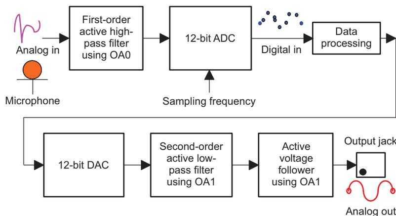
**Figure 4. Analog Signal Chain of MSP430 MCU**
