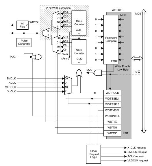
Figure 1-1. Watchdog Timer Block Diagram
