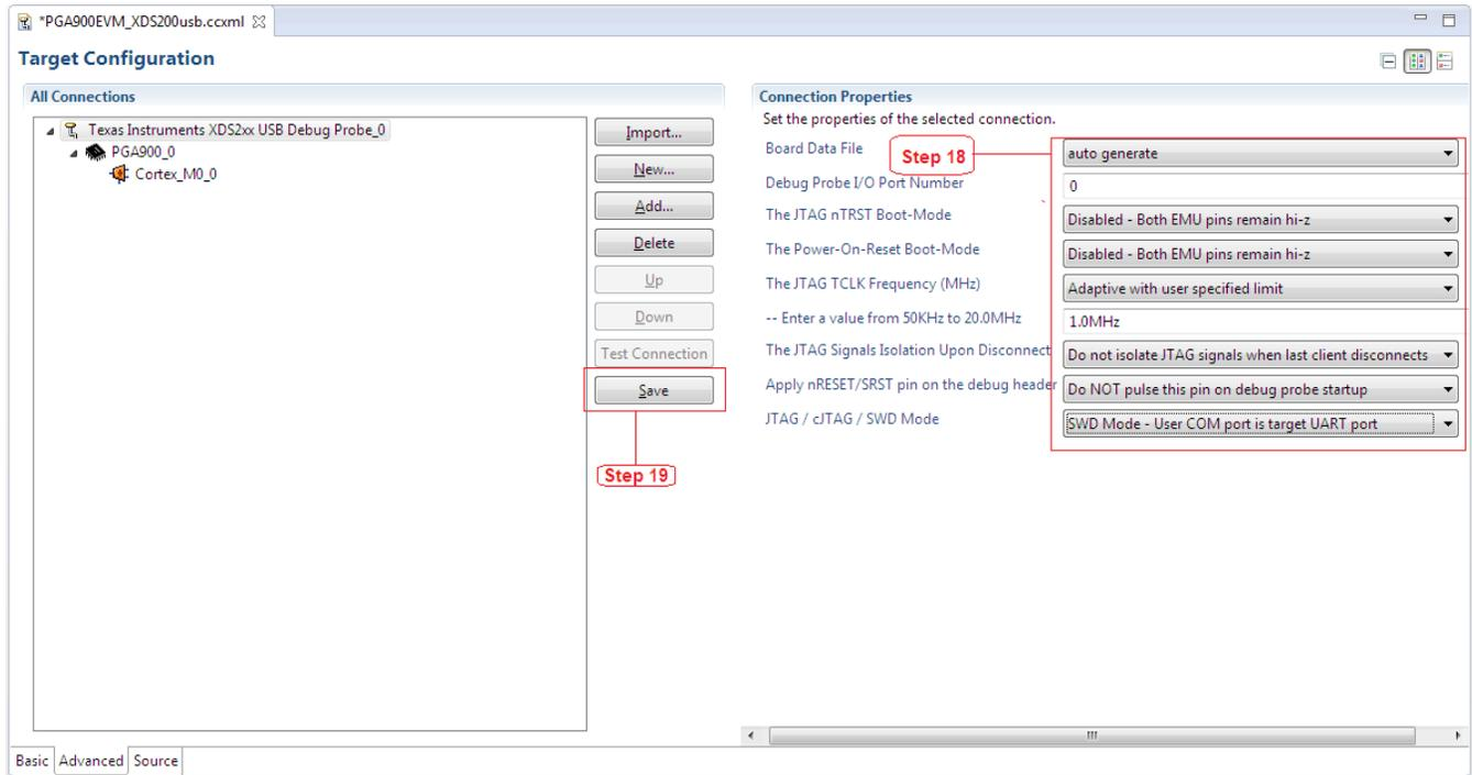
Figure 15. XDS200 USB Emulator Connection Properties
