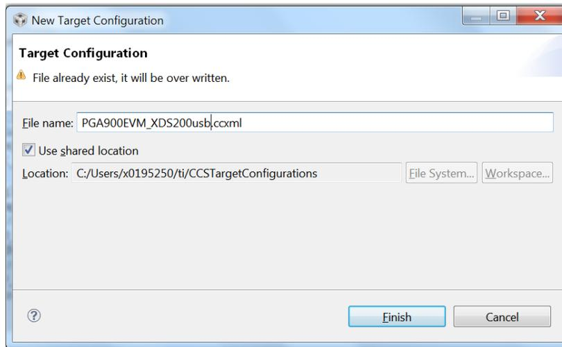
Figure 11. XDS200 Emulator Target Configuration
