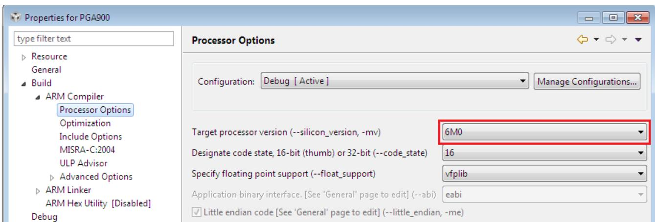
Figure 6. Target Processor Cortex M0 Selection
