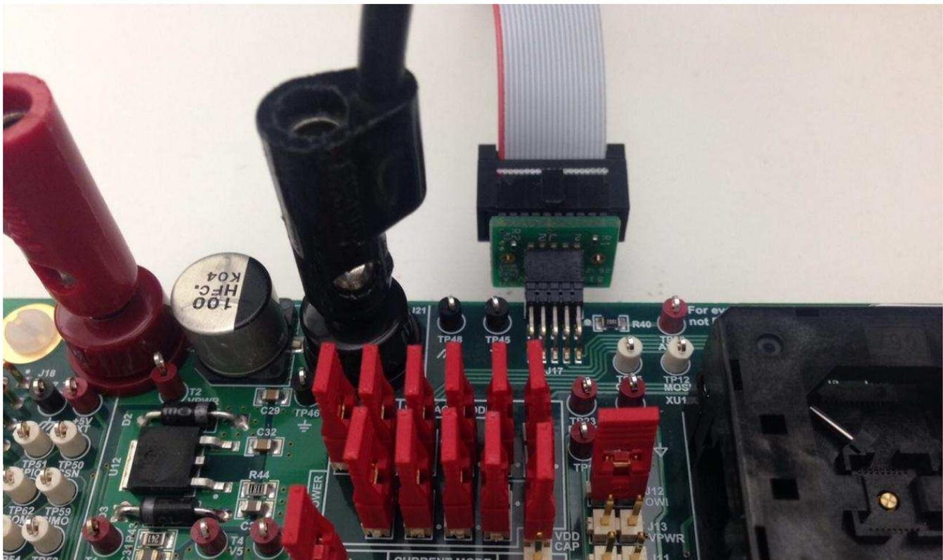
**Figure 10. XDS200 Emulator Connection to the PGA900EVM**
