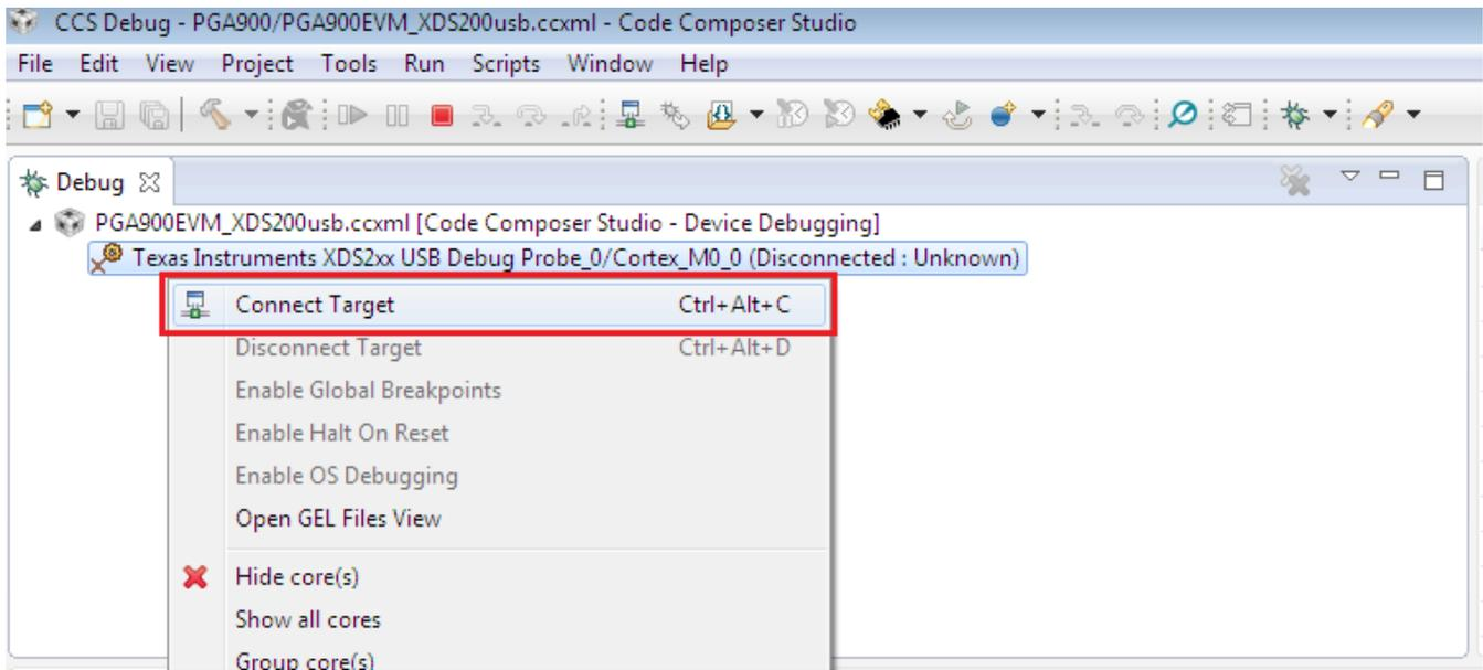
**Figure 20. Connect to the PGA900EVM**
