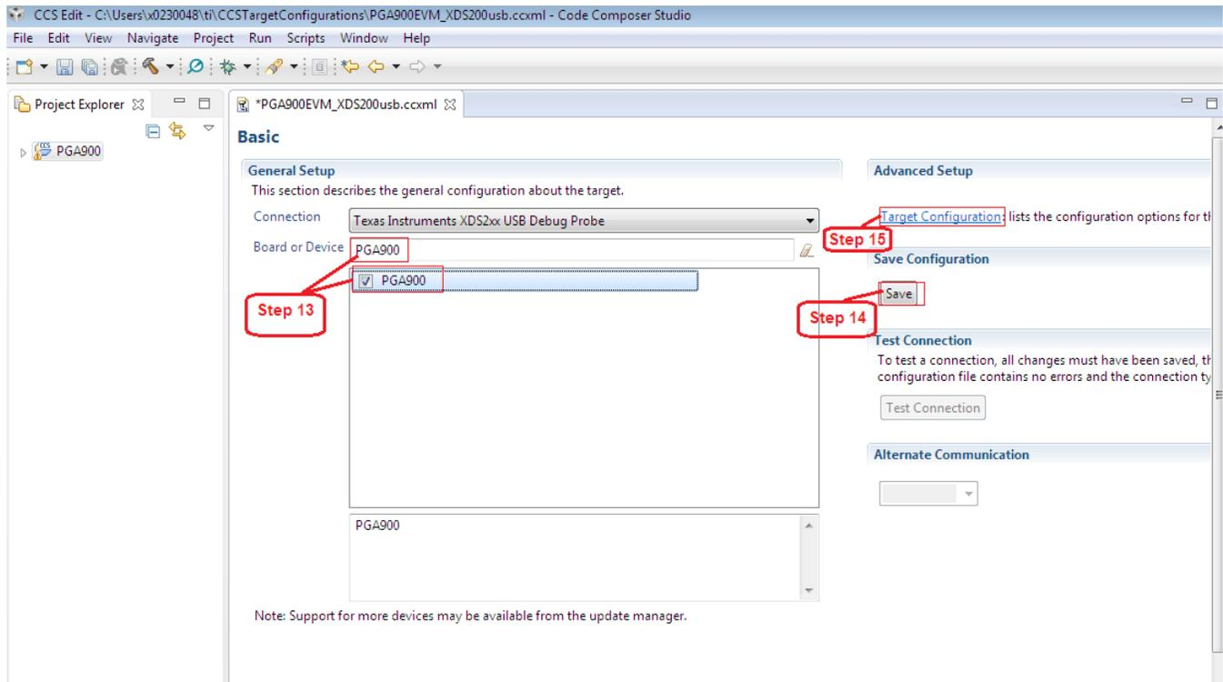
Figure 13. XDS200 Emulator Device Configuration
