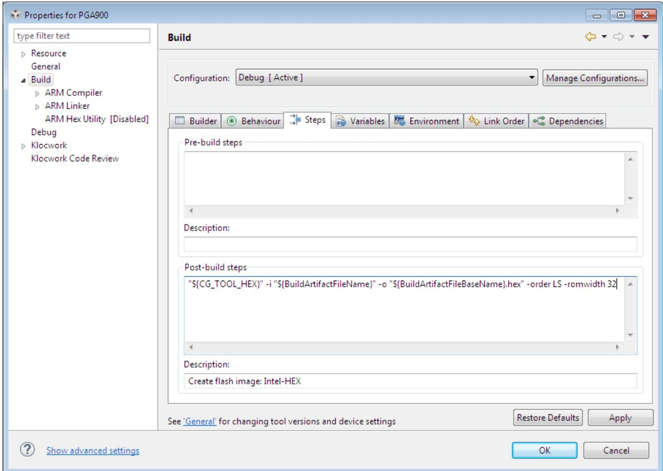
**Figure 9. Flash Image Intel Hex Configuration**
