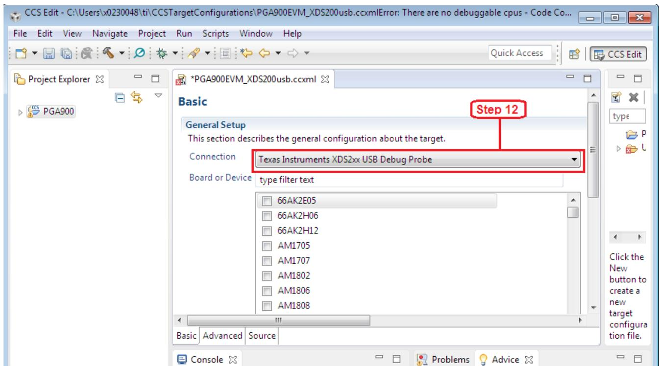
Figure 12. XDS200 Emulator Connection Configuration
