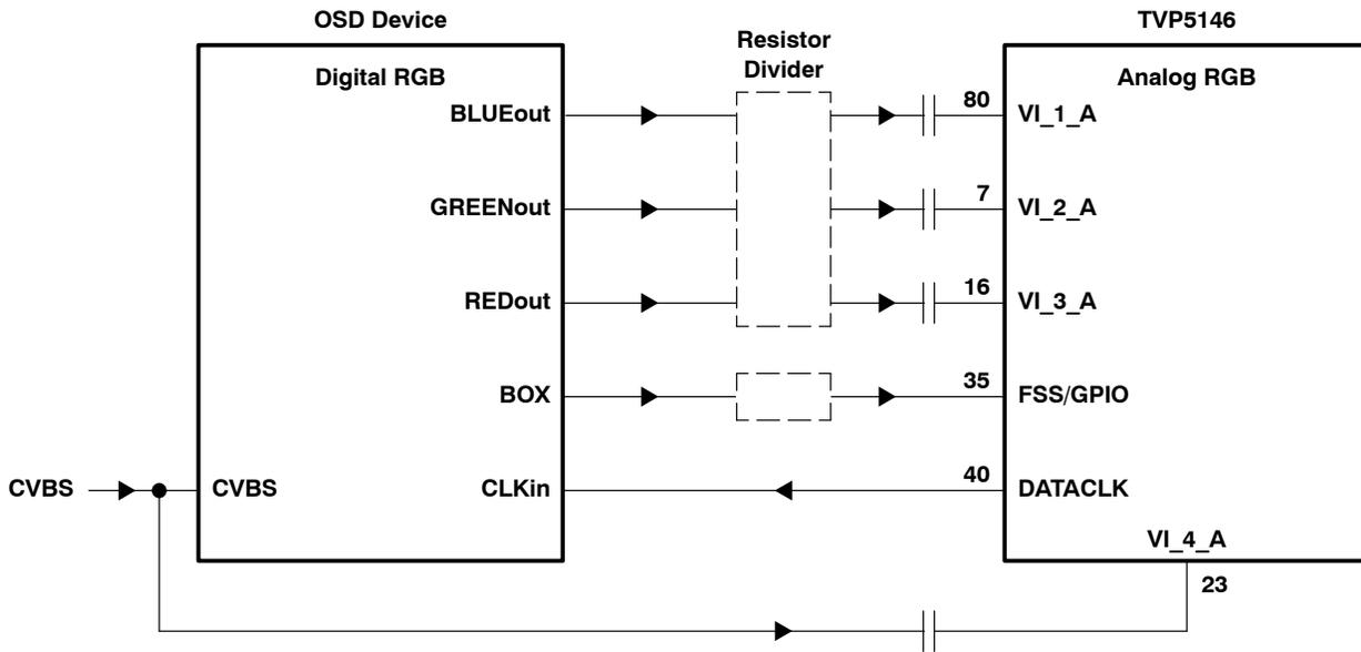
**Figure 7. SCART-Mode Overlay of Digital RGB**
