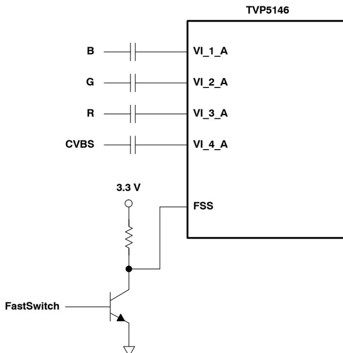
Figure 3. Typical RGB, CVBS, and FSS Connections for SCART
