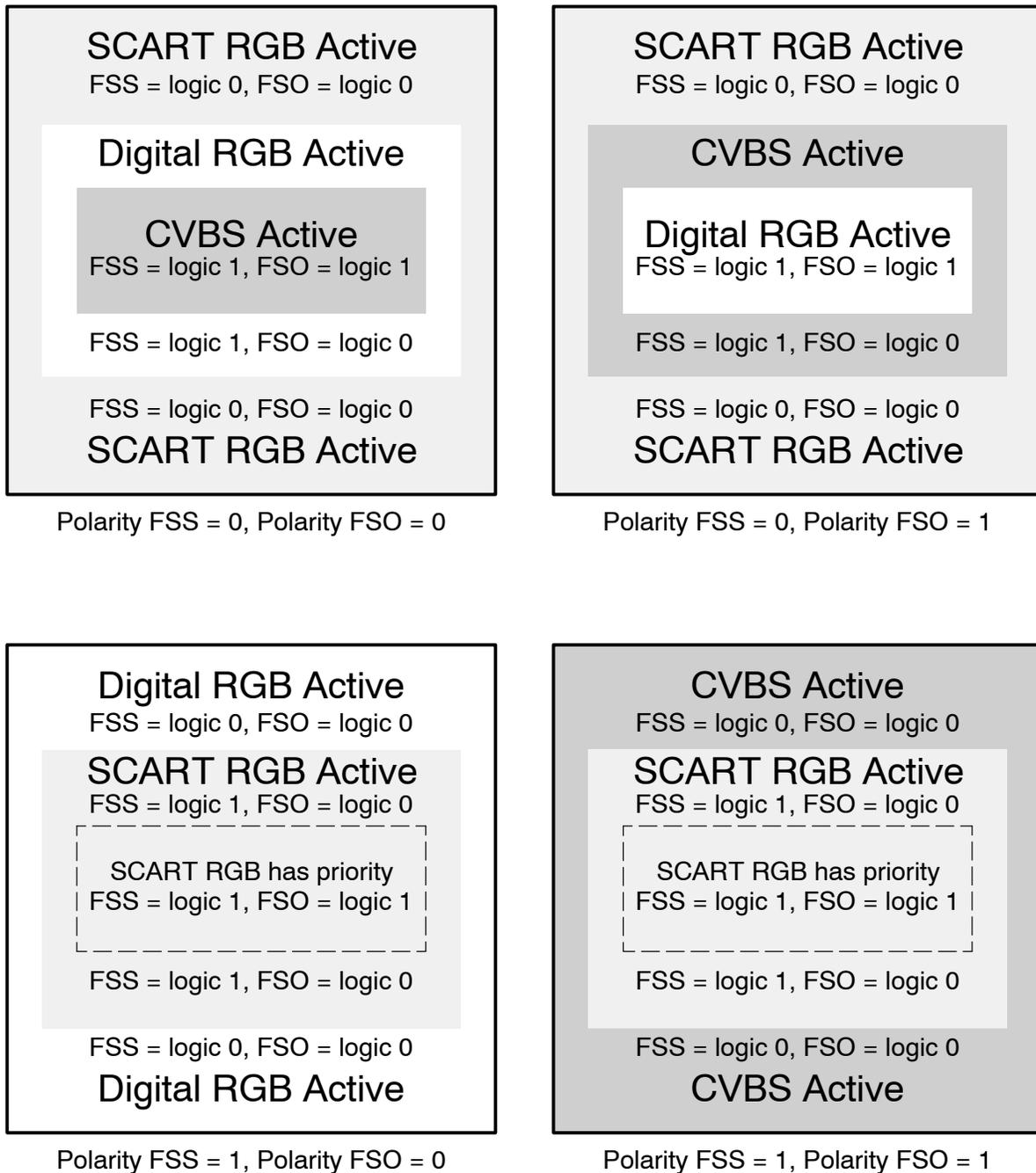
**Figure 9. Fast Switch Mode 004 [(CVBS ↔ Digital Overlay) ↔ SCART]**
