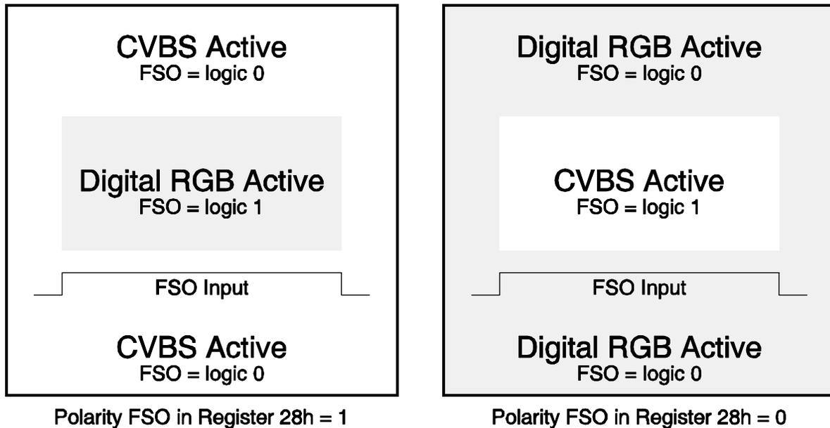
**Figure 4. Digital RGB Overlay with CVBS (Mode 001: (CVBS, S\_VIDEO ↔ Digital Overlay))**
