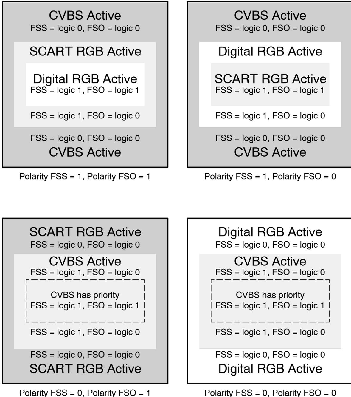
**Figure 10. Fast Switch Mode 005 [CVBS ↔ (SCART RGB ↔ Digital Overlay)]**
