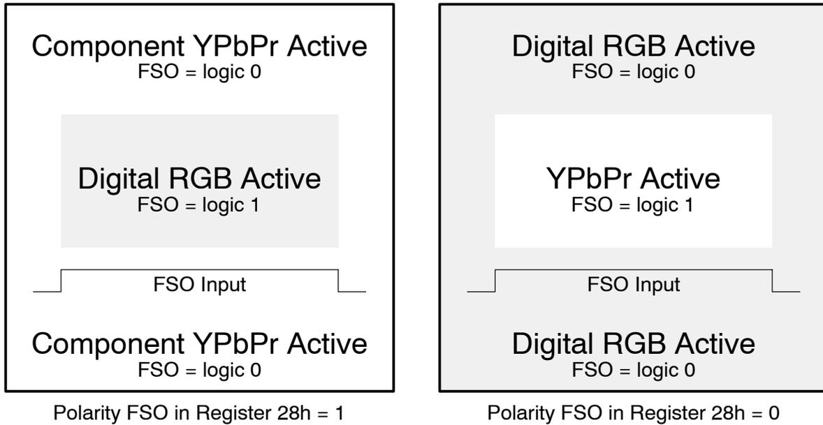
**Figure 5. Digital RGB Overlay With Component YPbPr (Mode 2: Component ↔ Digital Overlay)**
