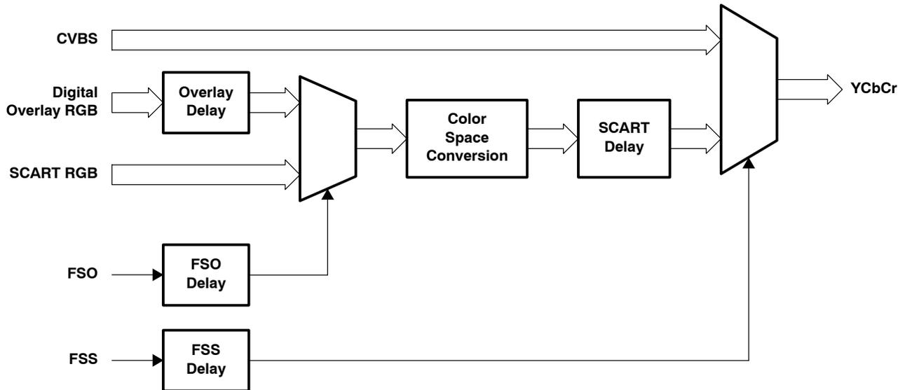
Figure 1. Fast-Switch Control of SCART and Digital Overlay
