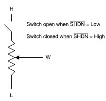
Figure 18. Equivalent Circuit for Shutdown Mode
