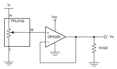
Figure 33. Digital to Analog Converter Schematic
