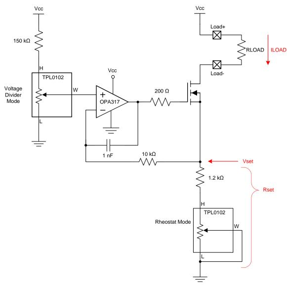
Figure 35. Variable Current Sink Schematic
