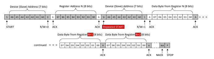
Figure 28. Read Operation from Multiple Registers
