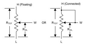
Figure 21. Equivalent Circuit for Rheostat Mode with Terminal L to Terminal W Resistance
