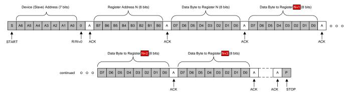
Figure 26. Write Operation to One or Multiple Registers
