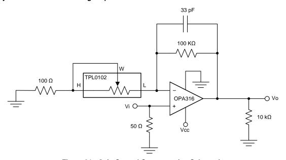
Figure 31. Gain Control Compensation Schematic
