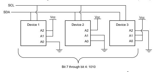
Figure 30. Examples of Device Address Configuration on I<sup>2</sup>C Bus
