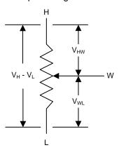
Figure 19. Equivalent Circuit for Voltage Divider Mode
