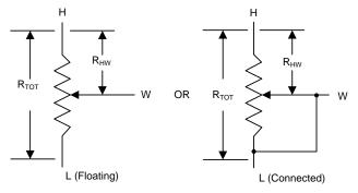
Figure 20. Equivalent Circuit for Rheostat Mode with Terminal H to Terminal W Resistance
