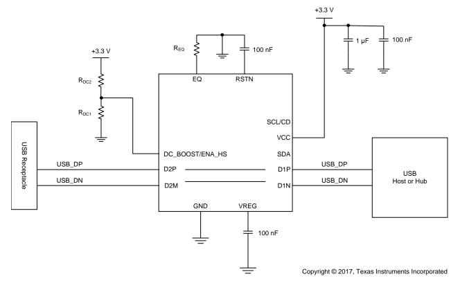
Figure 1. Reference Schematic
