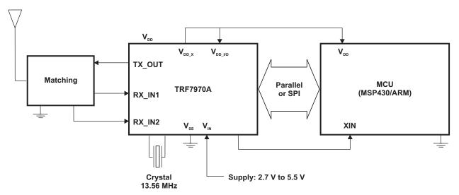
Figure 2. TRF7970A Embedded System Block Diagram
