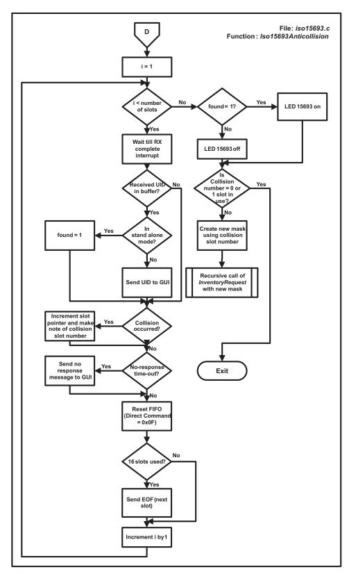
Figure 8. ISO15693 Anticollision Method Flow Chart (2)
