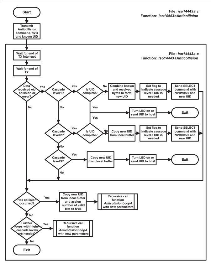
Figure 9. ISO14443A Anticollision Method Flow Chart
