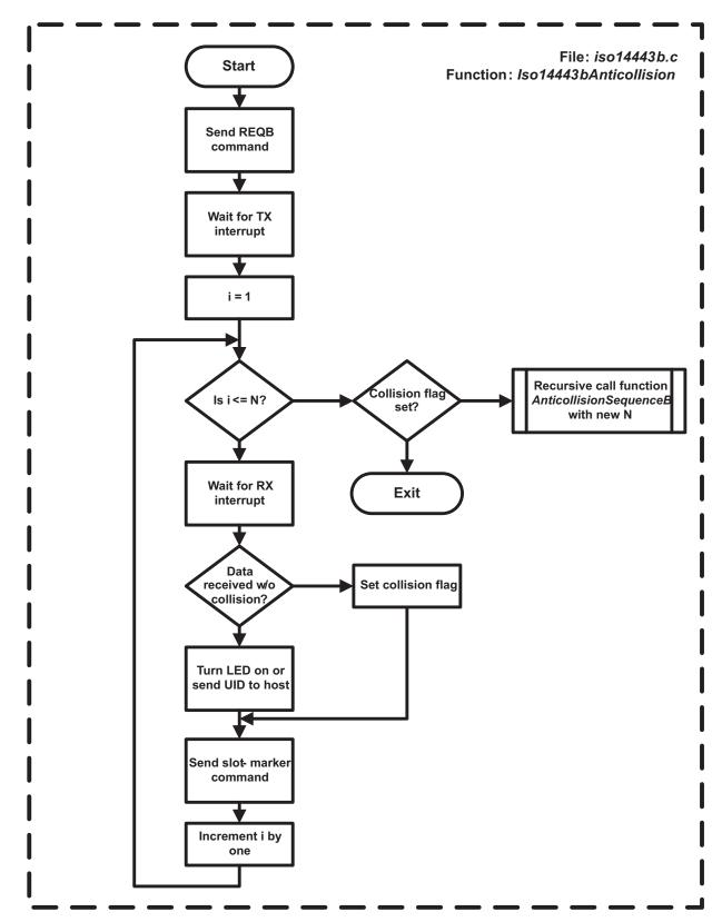
Figure 10. ISO14443B Anticollision Method Flow Chart
