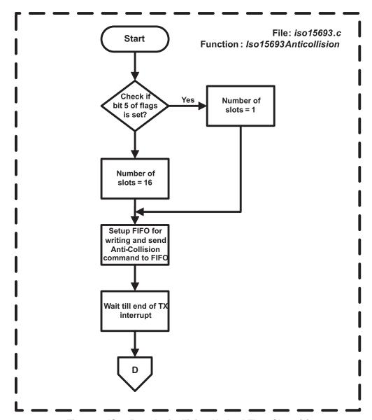
Figure 7. ISO15693 Anticollision Method Flow Chart (1)
