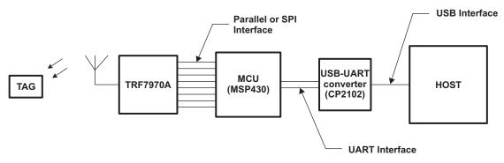
Figure 1. TRF7970A EVM Application Block Diagram
