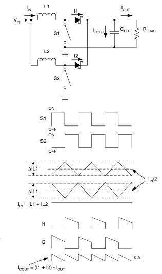
Fig. 2. Interleaved boost stage.
