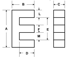
Fig. 12. Mechanical drawing of Mag-Inc EE core.
