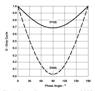
*Fig. 4. Duty cycle variation in universal PFC pre-regulator.*
