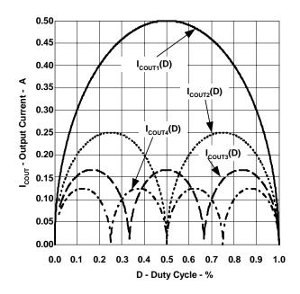
Fig. 13. Output capacitor RMS current.
