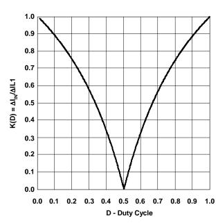
Fig. 3. Input ripple current reduction.
