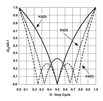
*Fig. 10. Ratio of input ripple current/inductor ripple vs. duty cycle (D).*
