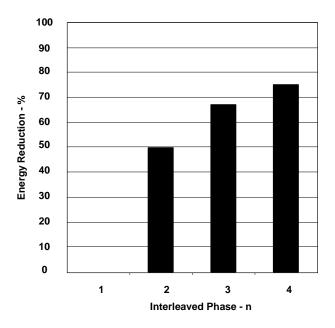
*Fig. 11. Percent of total inductor energy reduction.*
