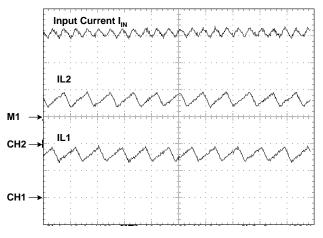
Fig. 7. Inductor ripple current,  $P_{OUT} = 350 W$ .
