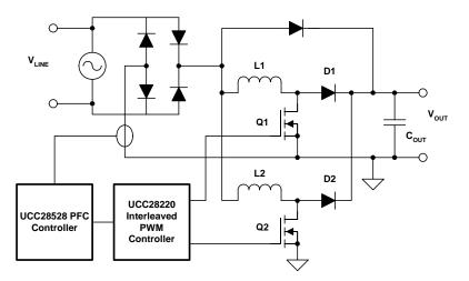
Fig. 6. Dual interleaved PFC.
