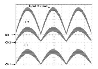
Fig. 8. Input current at  $V_{IN} = 85 V$ , 2 A/Div.
