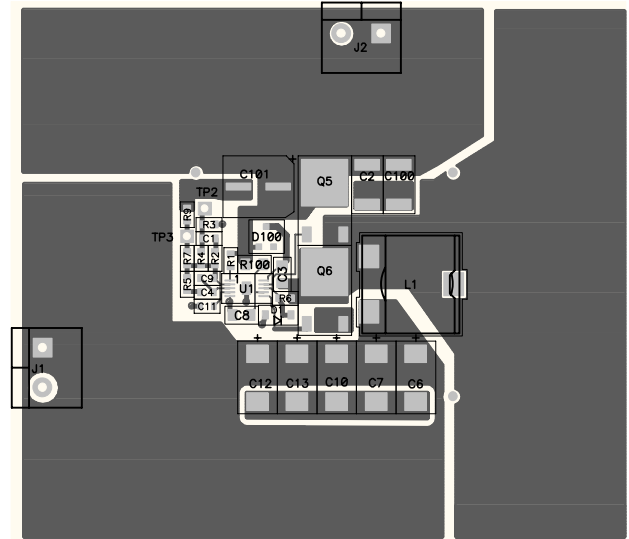
Fig. 34. Massive copper pours help spread heat.
