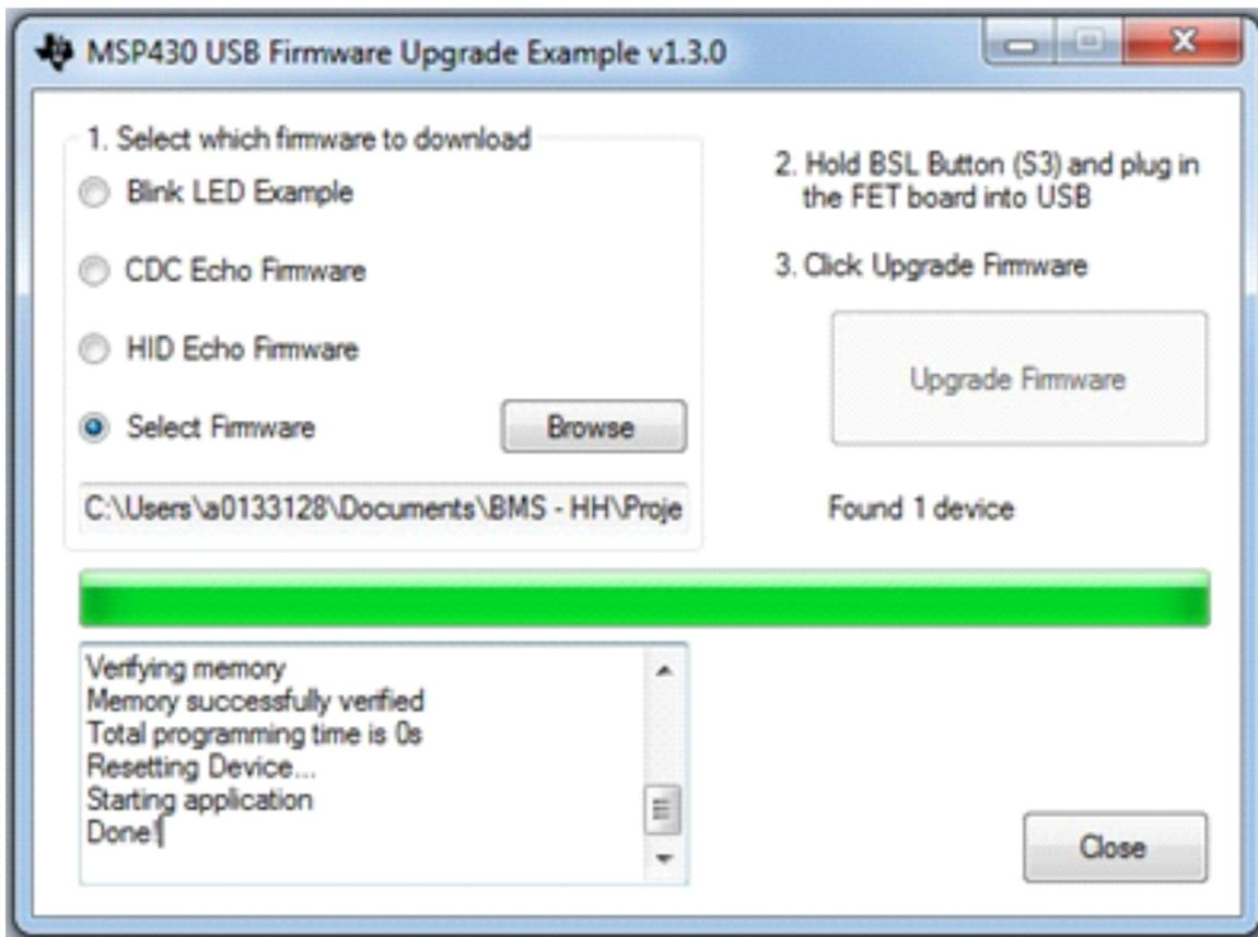
**Figure 12. MSP430 USB Firmware Upgrade Example—Successful FW Update**
