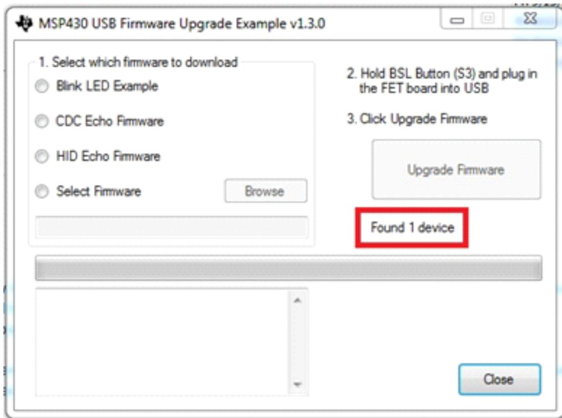
**Figure 11. MSP430 USB Firmware Upgrade Example Software**
