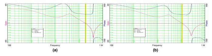
Figure 2. TPS62097 Closed-Loop Frequency Response Using a (a) 22-µF and (b) 2 x 22-µF Output Capacitor
