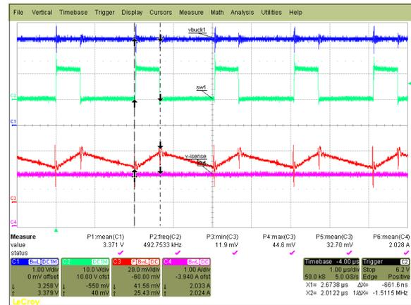
Figure 9. Case 2: Measurement With DC load — 2 A
