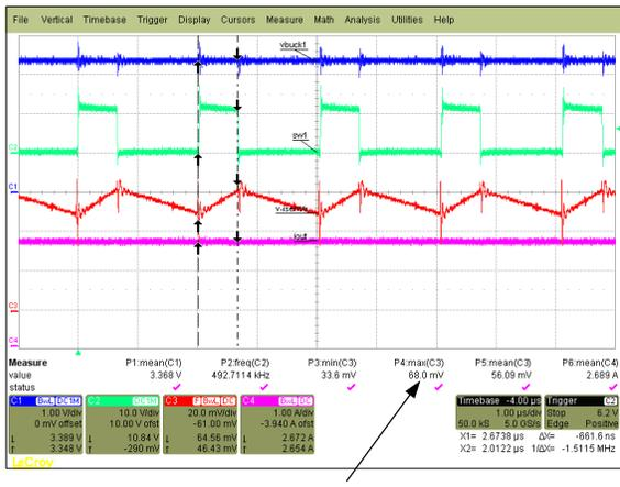
Device detects OC at around 68 mV
