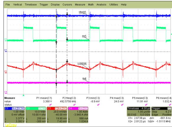
Figure 7. Case 2: Measurement with DC load — 1 A
