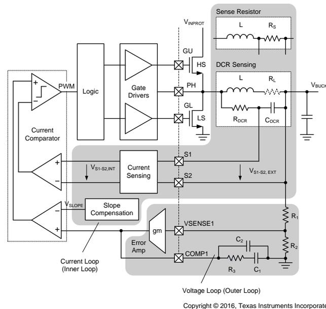
**Figure 1. BUCK1 Block Diagram With Current Sensing Using Inductor Resistance- $R_L$  or External Sense Resistor- $R_S$**
