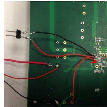
Current-sense resistor was removed, traces were cut.  $R_{DCR}$  and  $C_{DCR}$  were introduced.
