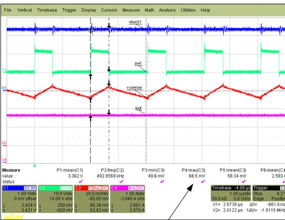
Device detects OC at around 68 mV
