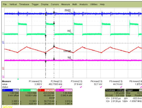
Figure 8. Case 1: Measurement With DC load — 2 A
