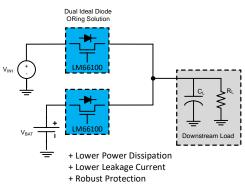
Figure 1. Typical ORing Application
