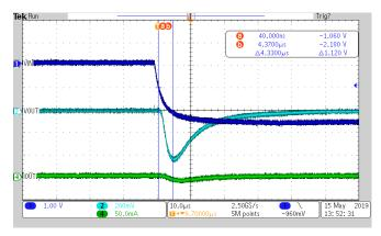
**Figure 6. Reverse Polarity Protection**
