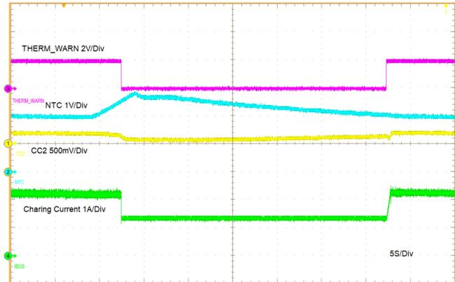
Figure 13. Active Current Limit In Type-C Port
