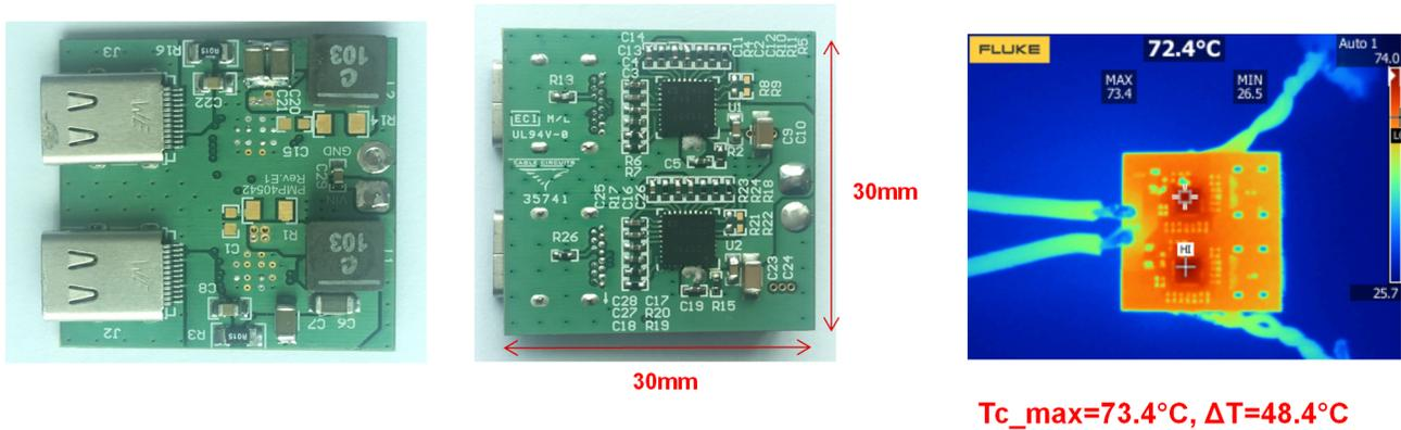
Figure 6. Dual Type-C Port PCB View and Thermal Performance
