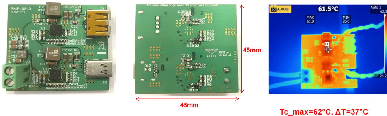
Figure 8. Type-A And Type-C Dual Port PCB And Thermal
