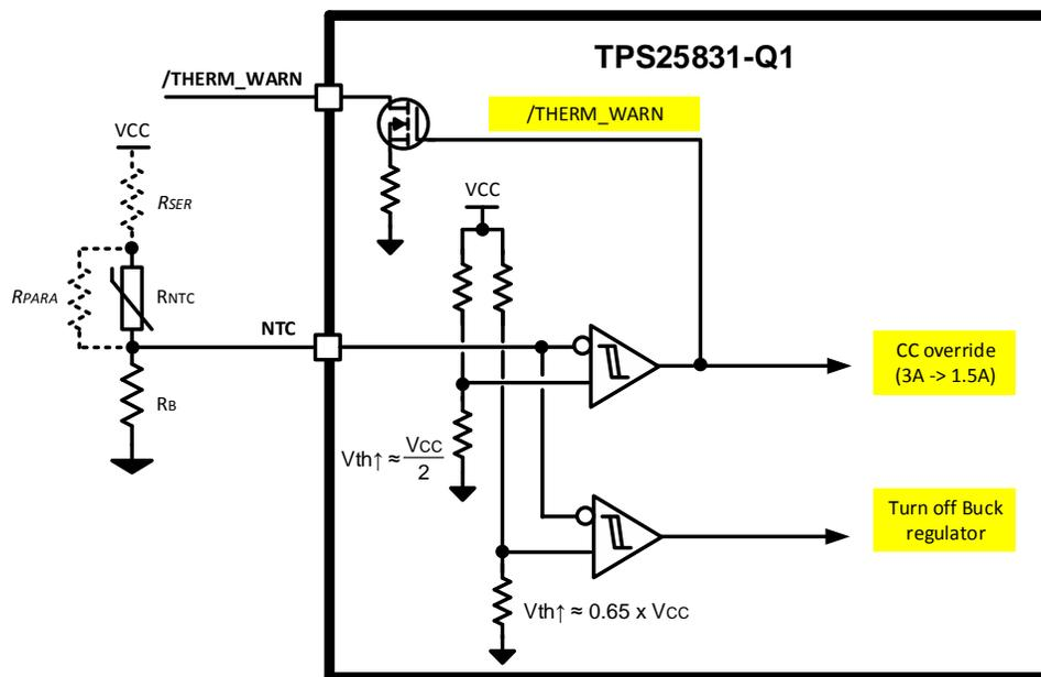
Figure 9. NTC Input Pin
