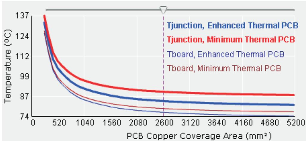
**Figure 2. Example Graph Showing Junction Temperature as a Function of Spreading Plane Area for the TPS25831-Q1 Device at 0.5 W with 65°C Ambient Temperature**
