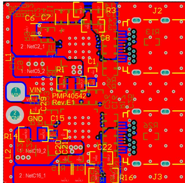
Figure 4. PMP40542 Top View
