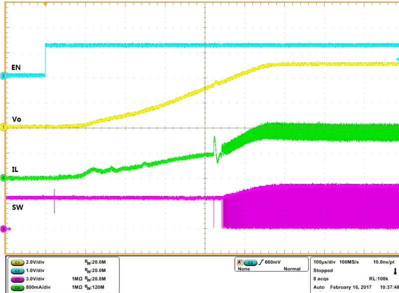
Figure 1. Startup Waveforms ( $R_{load} = 5 \Omega$ )
