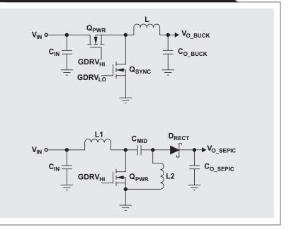
the SEPIC converter uses  $Q_{\rm PWR}$  only to charge the inductor. During this time the output capacitor must supply the battery-charging current. When  $D_{\rm RECT}$  turns on, the now charged inductor provides both the output capacitor recharging and battery-charging currents. Hence, the SEPIC converter's output-voltage ripple will always be
