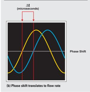
Coriolis acceleration acting in opposite directions on either side of the tubes and the fluid's resistance to the vertical motion. Sensor electrodes placed on both the inlet and outlet sides pick up the time difference caused by this motion. This phase shift due to the twisting forces is a direct measurement of mass flow rate. Figure 4 shows typical detection results.
