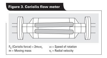
tubes. When the fluid starts flowing through the tubes, it is subject to Coriolis force. The oscillatory motion of the tubes superimposes on the linear motion of the fluid, exerting twisting forces on the tubes. This twisting is due to
