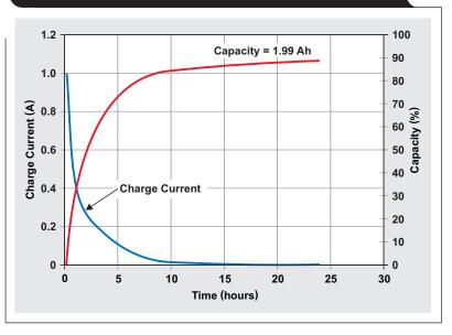
charging time and was used to determine that  $\sim 2$  Ah were delivered to the cell. Figure 6 shows the discharge profile of the pack after it was charged without termination. The pack's measured capacity was 1.99 Ah.
