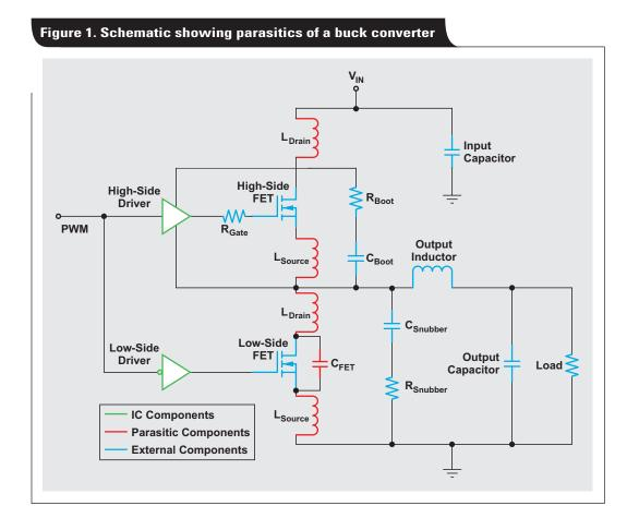
cycle, the converter prepares to switch the low-side FET off and the high-side FET back on to replenish power to the output L.
