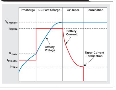
complete charge cycle at a 1-A (1C) constant-current (CC) fast charge.
