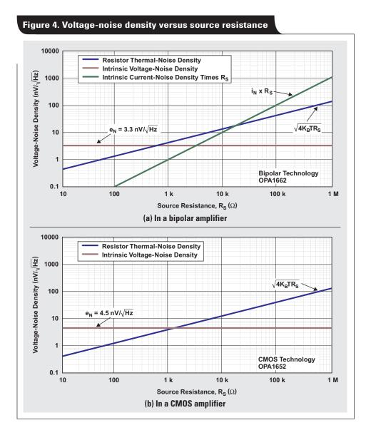
total noise density for the CMOS amplifier is given by Equation 2:
