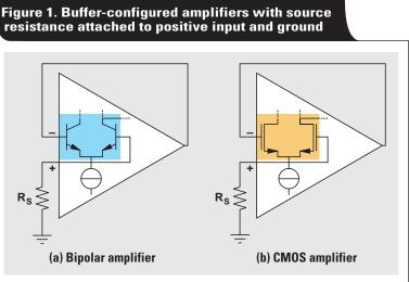
$$E_{O} = \sqrt{\left(e_{N}\right)^{2} + \left(i_{N} \times R_{S}\right)^{2} + \left(4K_{B}TR_{S}\right)}$$
