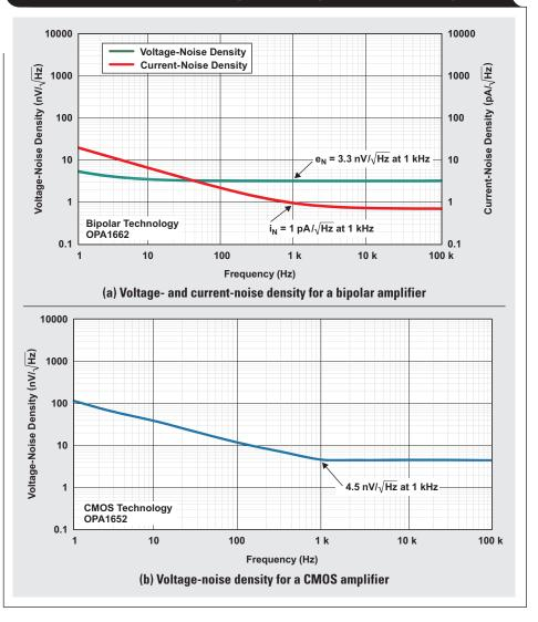
amplifier, and the first and third terms for the CMOS amplifier. The sweeping variable in Equation 1 is the source resistance. In other words, the voltage-noise density is calculated as a function of source resistance with voltage- and current-noise densities taken at 1 kHz. This is shown in Example 1 for a bipolar amplifier.
