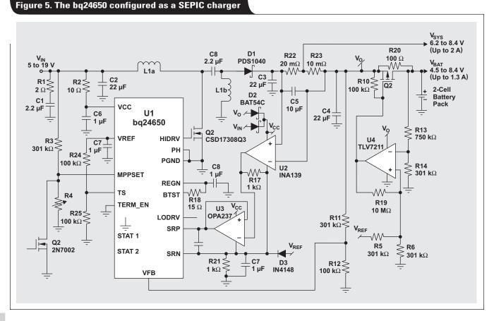
if two separate inductors had been used. R18 was used to slow down the fast turn-on of Q1. Also, the controller's PH pin was grounded to help provide the boosted output voltage. A
