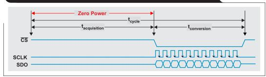
Different data converters will require different approaches to adjust the timing. The most common device type has an internal clock that sets the conversion time. Regardless of cycle time, the conversion phase will always remain the same length of time. Increasing the acquisition time in these device types requires a decrease in the operating sampling rate. A constant conversion phase will result in a longer cycle time dominated by the acquisition phase.
