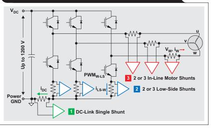
over one pulse-width modulation (PWM) cycle for each shunt placement. From a system view, the motor in-line shunts offer major performance advantages, while from an amplifier view, the low-side shunts enable lower-cost solutions, as shown in Table 1 on the next page.
