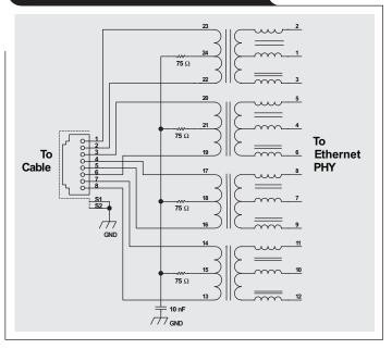
To create the ability to inject power, Figure 1b shows that adding one capacitor per middle tap interrupts the DC path. Since the DC path is no longer shorted, a DC voltage can be applied symmetrically between each differential pair. In total, it is possible to have up to four pairs of twisted cable. These pairs go to the powered-device (PD) controller over two rectifier bridges. By using a rectifier, the polarity as well as the pairs used does not matter.
