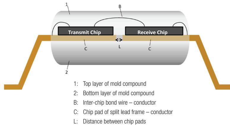
**Figure 2.** Depicted is the internal structure of a two-chip digital isolator.
