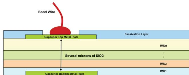
**Figure 5.** High-voltage capacitor with multiple layers of inter-metal dielectric.
