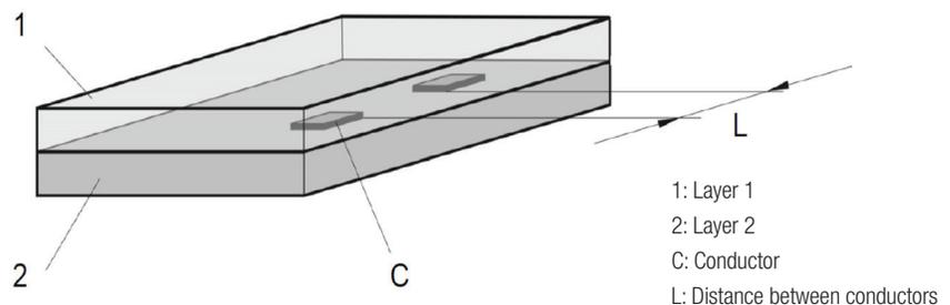
**Figure 1.** Illustrated is the distance between conductors on an interface between two layers (Source: IEC 61010-1 edition 3.0, sub-clause 6.7.2.2.2\*)
