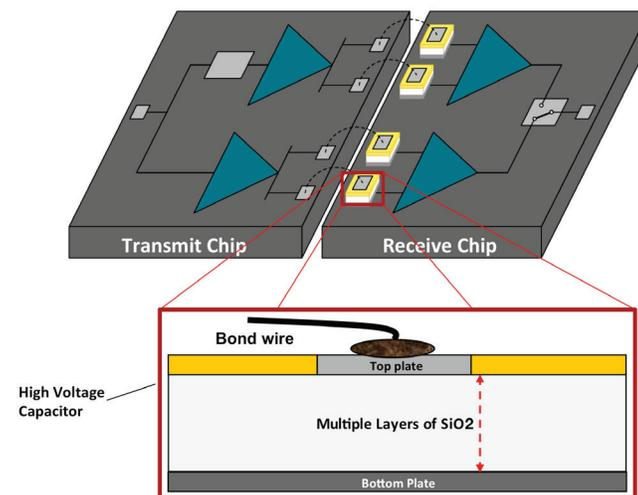
**Figure 3.** An integrated high-voltage capacitor is the main source of isolation.
