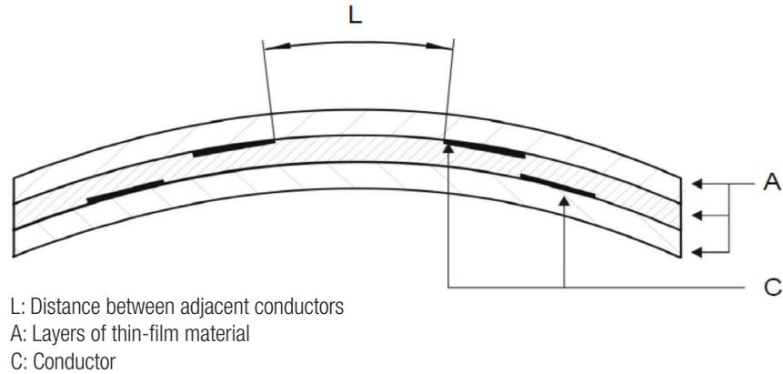
**Figure 4.** The distance between conductors located between the same two layers
