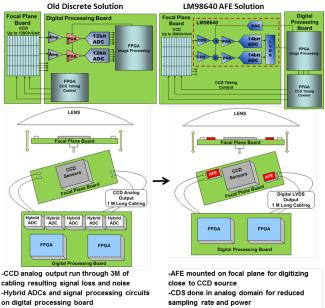
cabling resulting signal loss and noise -Hybrid ADCs and signal processing circuits on digital processing board -ADC run at 2X pixel rate and CDS done in digital domain on FPGA -ADC parallel output requiring more FPGA I/O pins
