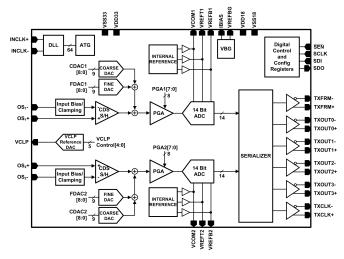
Figure 2. LM98640 Block Diagram
