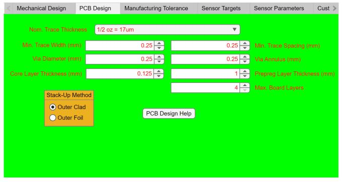
Figure 5-7. LDC5072 Sensor Designer PCB Design Tab
