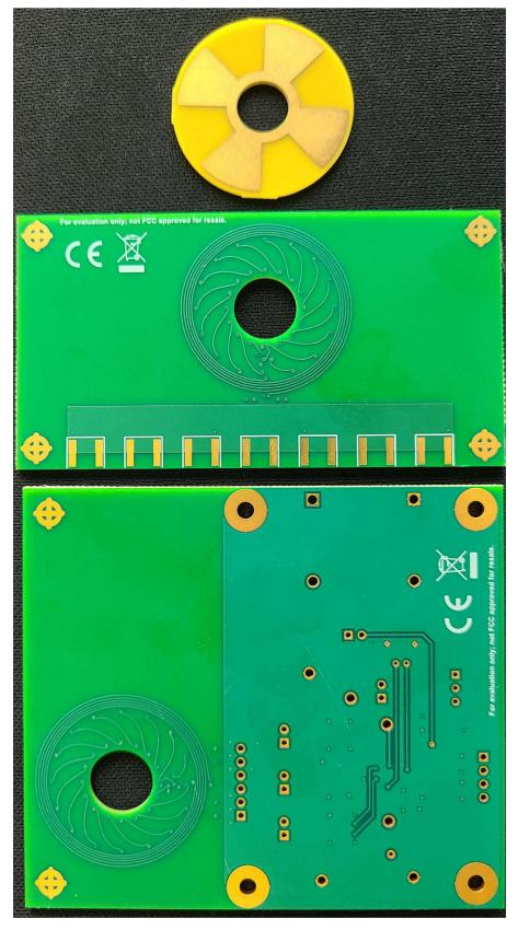
Figure 8-2. Underside of Sensor, LDC5072 and Target PC boards created by the LDC5072 Sensor Design Tool
