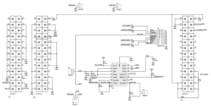
Figure 12. LM1000 AVS System Controller Schematic
