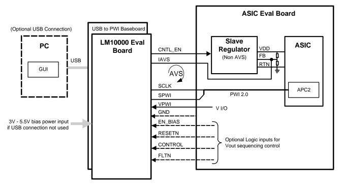
Figure 4. In Situ PowerWise® AVS Setup (Closed Loop Voltage Scaling)
