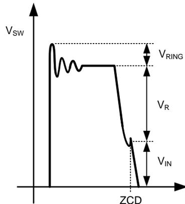
**Figure 19. Switch Node Ringing**
