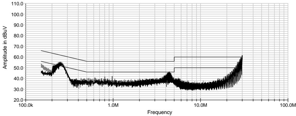
Figure 7. 120V 15W Conducted EMI Peak Scan
