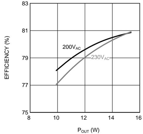
**Figure 3. 230V 15W Version Efficiency vs. Output Power**
