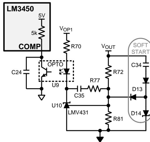
Figure 16. Secondary Error Amplifier Circuit
