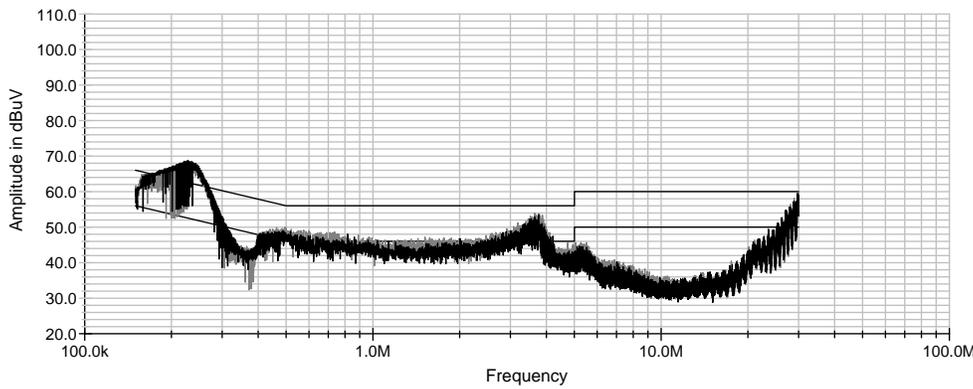
Figure 8. 230V 15W Conducted EMI Peak Scan
