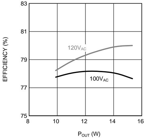
**Figure 2. 120V 15W Version Efficiency vs. Output Power**
