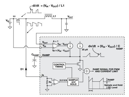
Figure 3. Emulated current mode control ramp generator.
