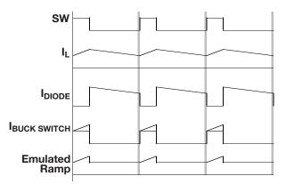
Figure 2. Buck regulator waveforms.
