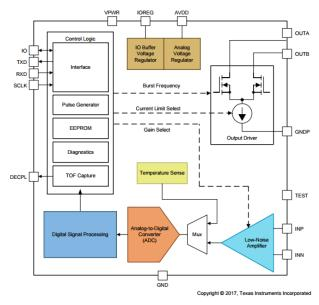
Figure 3. PGA460-Q1 Block Diagram
