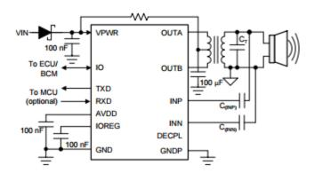
Figure 2. PGA460-Q1 Transformer Drive Schematic
