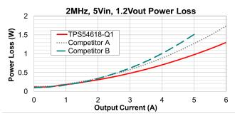
Figure 2. Power loss of the same devices as above
