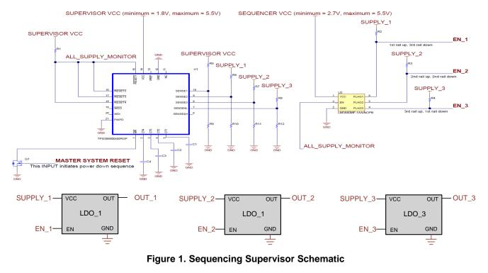
**NOTE:** The voltage regulators (LDO\_1, LDO\_2, and LDO\_3) can be replaced with pass PFETs and the EN\_1, EN\_2, and EN\_3 signals coming from the LM3880 can be used to control the gates of the pass PFETs if no voltage regulation is required.
