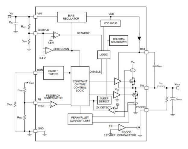
Figure 1-1. Functional Block Diagram
