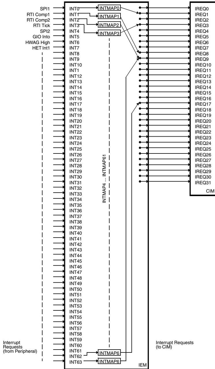
As illustrated in Figure 1, the IEM is used to map the interrupt requests from peripheral modules in the 470R1Vx system (INT[63:0]) to the CIM interrupt requests IREQ[31:0].
