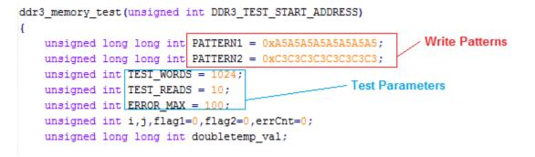
Figure 1. Variables That Can be Modified in the *ddr3\_memory\_test()* Function of the DDR3 Debug GEL
