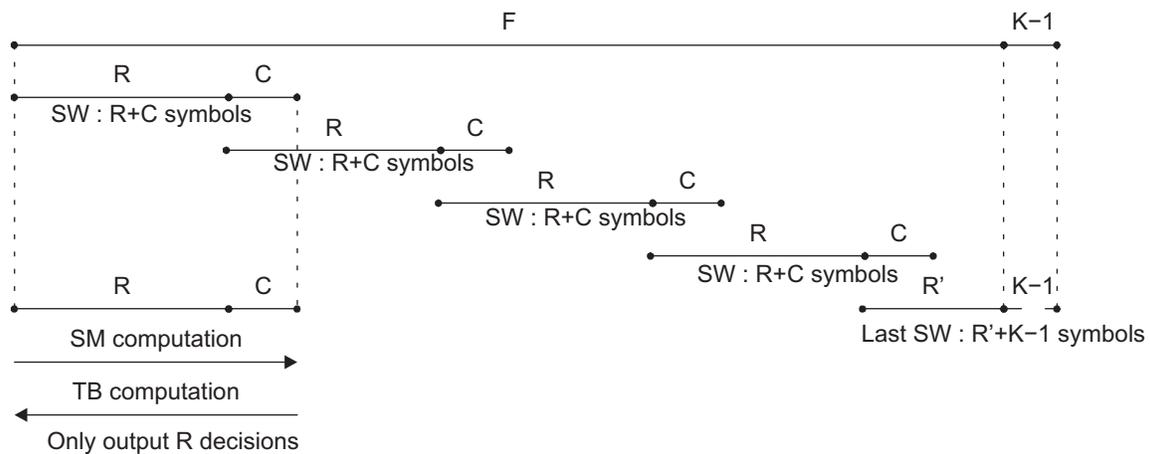
Figure 28. Convergent Traceback Mode-Example With Five Sliding Windows
