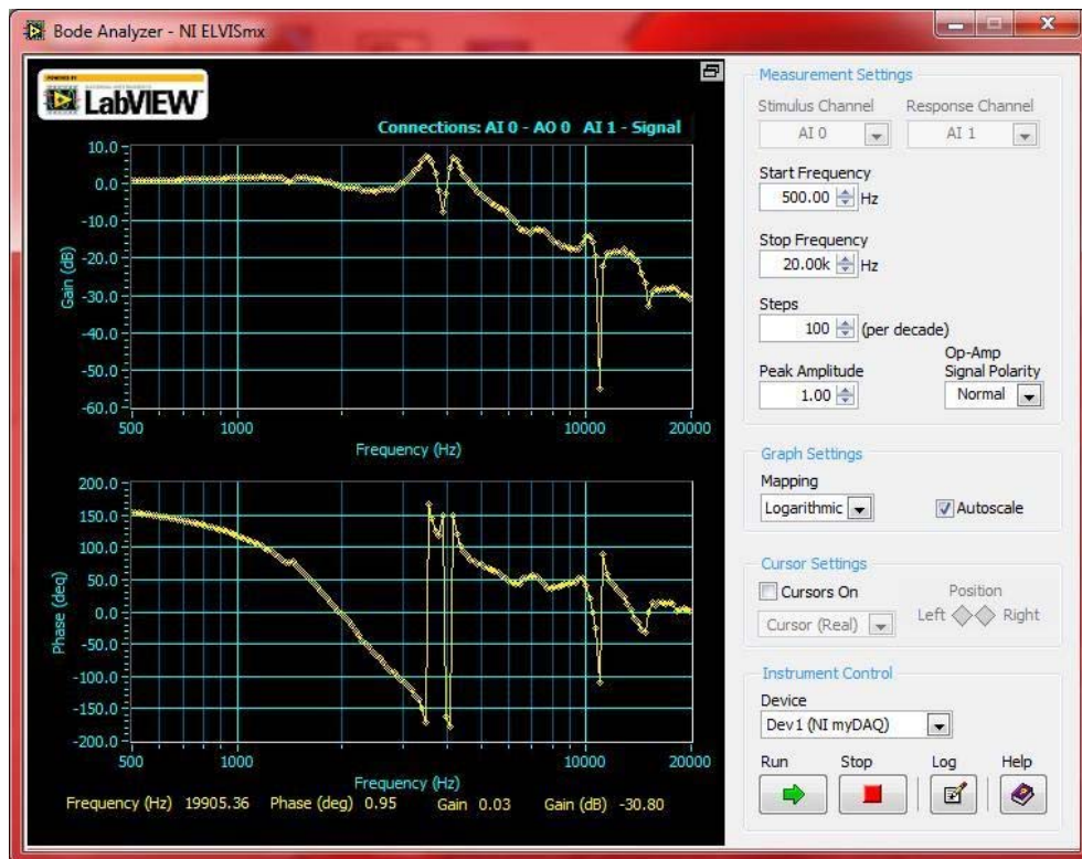
Figure 9: Frequency response of the included loudspeaker, measured by the microphone circuit.
