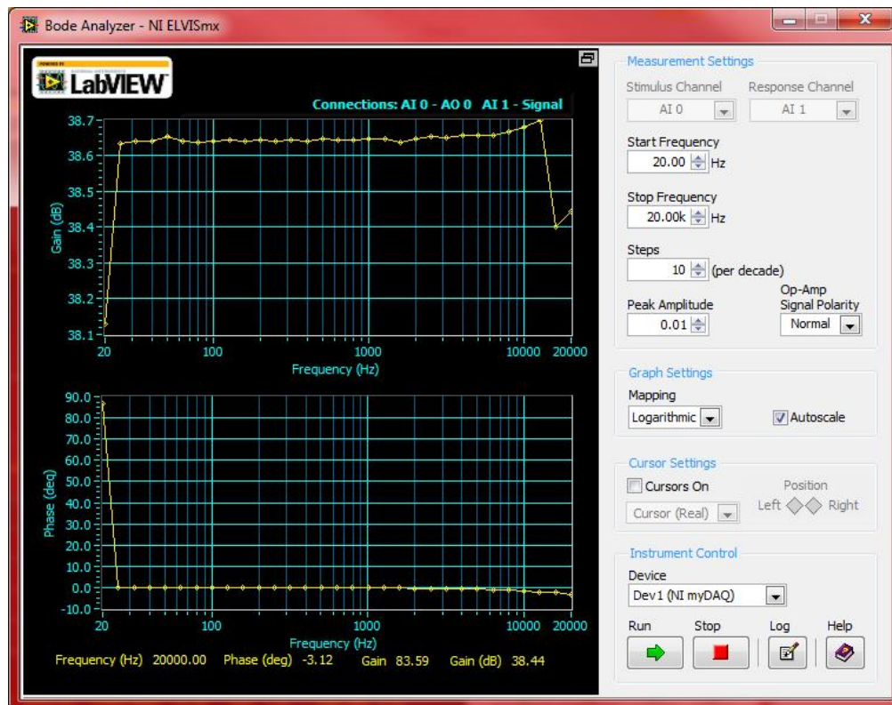
Figure 6: Real-world performance of the microphone amplifier circuit
