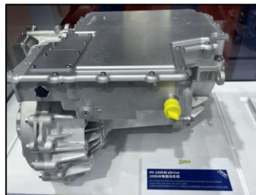
Inverter + Motor + Reducer
