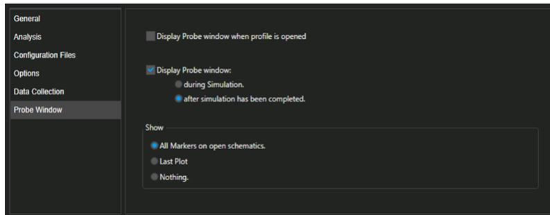
**Figure 7. Probe Window tab of the Simulation Settings dialog**
