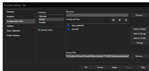
**Figure 3. Configuration Files tab of the Simulation Settings dialog**
