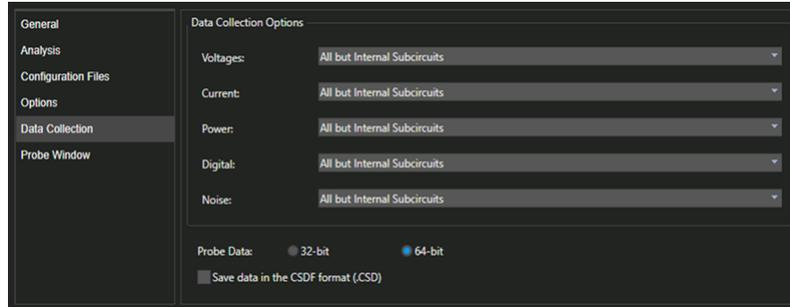
**Figure 5. Data Collection tab of the Simulation Settings Dialog**
