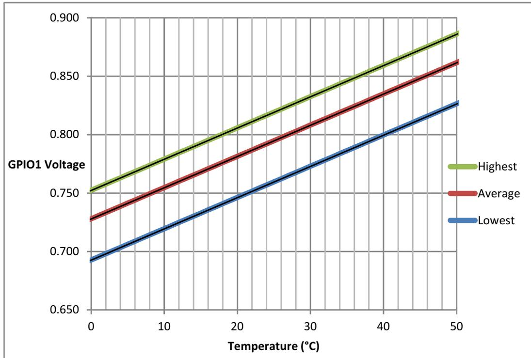
Figure 1. GPIO1 Voltage vs Temperature
