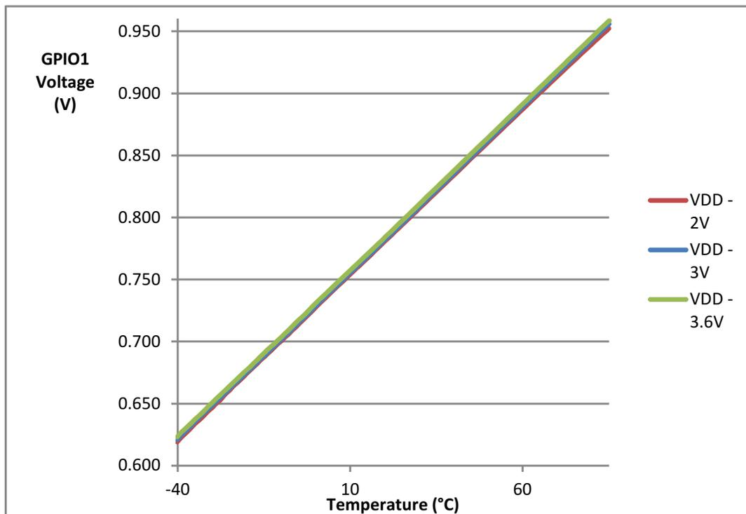
Figure 3. Typical GPIO1 Measurements vs Supply Voltage
