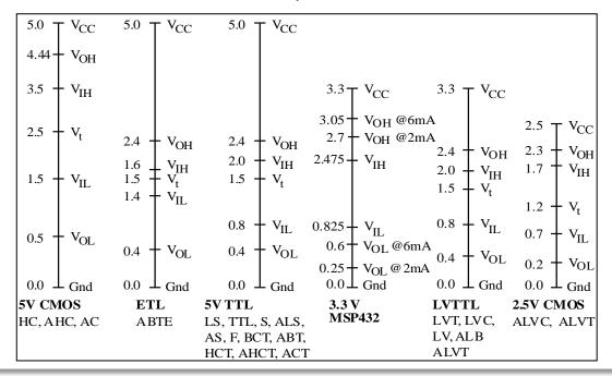
$V_{OL} \le V_{IL}$  for all inputs and  $V_{OH} \ge V_{IH}$  for all inputs  $I_{OL} \ge \sum I_{IL}$  for all inputs and  $I_{OH} \ge \sum I_{IH}$  for all inputs
