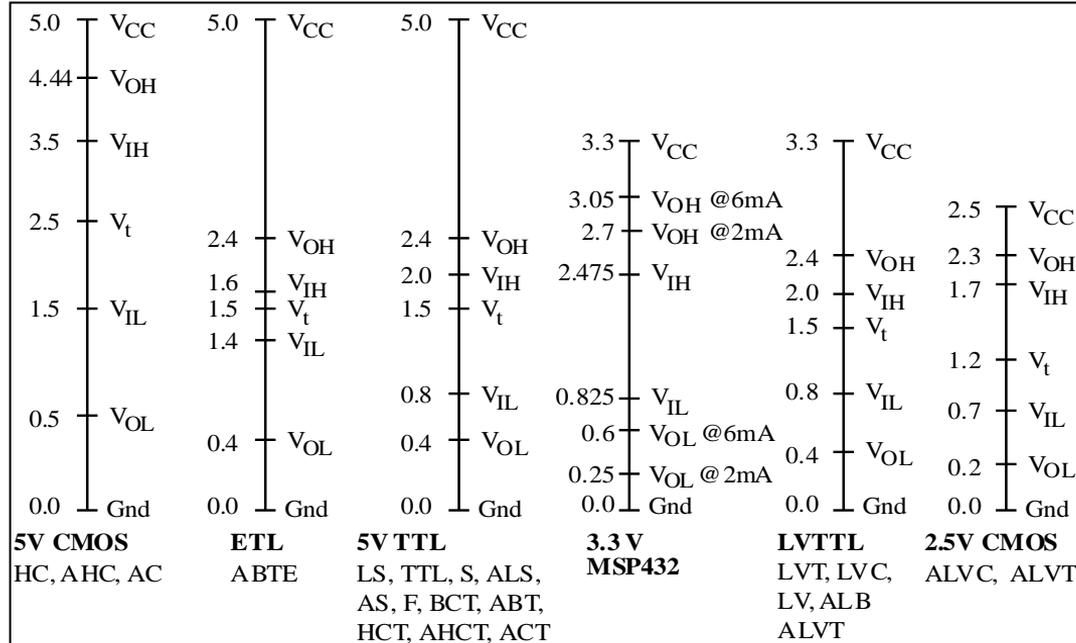
$$V_{OL} \leq V_{IL} \text{ for all inputs} \quad \text{and} \quad V_{OH} \geq V_{IH} \text{ for all inputs}$$
