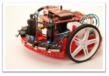
Figure 1. IR distance sensors, positioned at the front of the robot.
