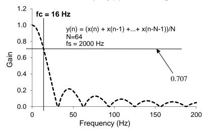
Figure 5. Frequency response of averaging filter with N=64.
