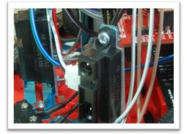
Figure 1. Three IR distance sensors positioned at the front of the robot.
