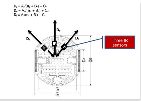
Figure 3. Define distance measured from a central point on the robot.
