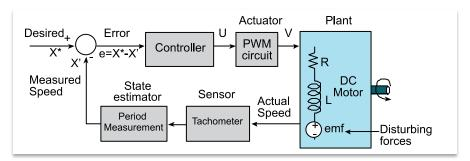
Figure 1. Block diagram of a MSP432-based closed-loop control system.
