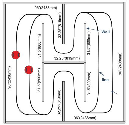
Figure 11. Create a robot explorer that races around a track with bump sensors and line sensors.
