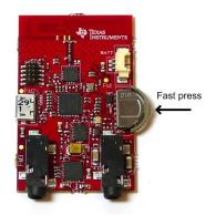
In the pre-programmed firmware the pairing button is mapped to pressing the rocker switch IN (not hold, which is power toggling as described in 4).
