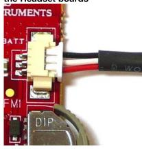
There's only one way to connect the battery plug to the socket on the board. With the pre-programmed firmware the CC8531 enters the OFF power mode when the battery is connected. The batteries should have enough charge out-of-the-box to establish a link and stream audio. To charge the battery, see section 9. With full battery the link should run for typically 15 hours, the Master being the bottleneck. The Slave plays audio for 22 hours typically.
