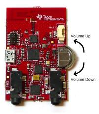
The pre-programmed Slave firmware is configured to have so-called "local volume control" meaning that the Slave controls its own volume locally. The volume buttons are mapped to clicking/holding the rocker switch UP and DOWN.
