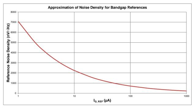
Figure 7. Characteristic Curve: Reference Noise vs Current
