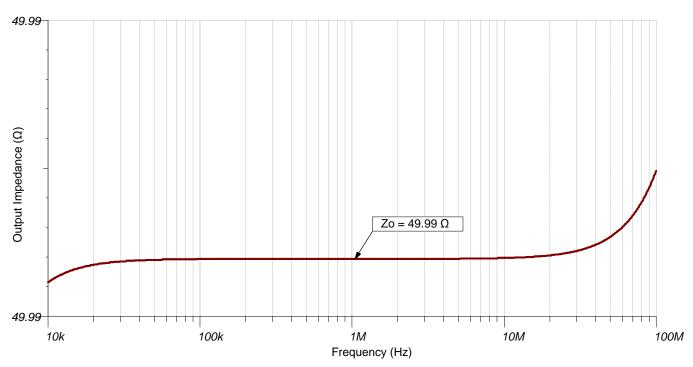
Figure 10. TINA-TI™ Simulation Result: Output Impedance of OPA350
