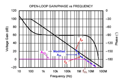
Figure 5. Analyzing Effect of RC-Filter on Op Amp Stability Using AoL Response
