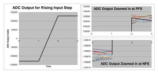
Figure 1. Measurement Data - ADC Transient Output Response for Rising Input Step
