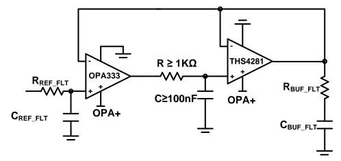
Figure 12. DC Equivalent Schematic of Reference Buffer
