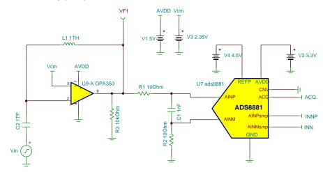
Figure 16. TINA-TI™ Schematic - Checking Input Amplifier Stability
