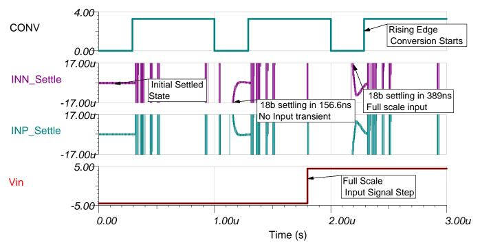
Figure 18. TINA-TI™ Simulation Result - ADC Input Settling
