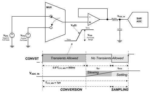
Figure 3. Timing Diagram For Input Stimulus
