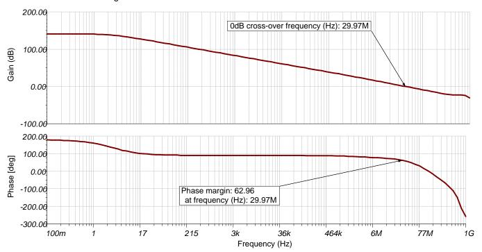
Figure 17. TINA-TI™ Simulation Result - Loop Gain Magnitude and Phase Plot for Input Driver Stability
