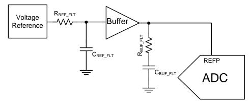
Figure 6. Simplified Schematic of Reference Driver Circuit
