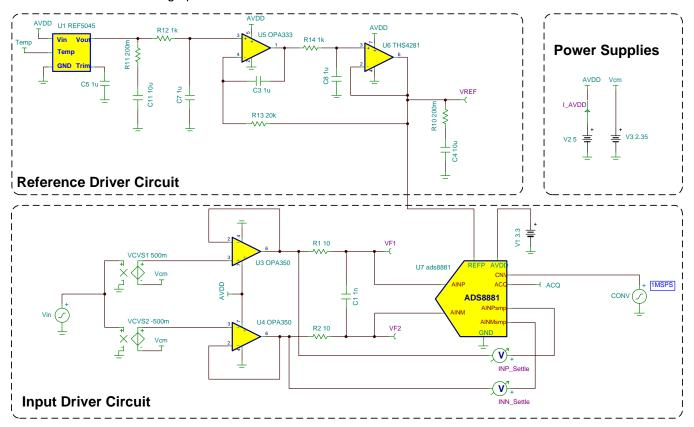
Figure 15. TINA-TI™ Schematic - Complete Data Acquisition Block
