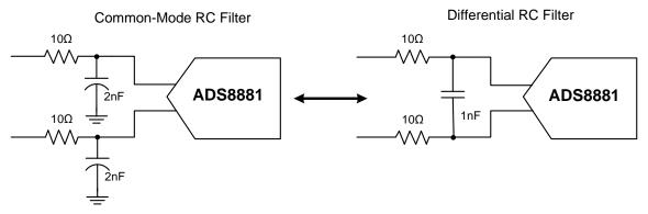
Figure 8. Design Configurations for Anti-aliasing RC-filter at ADC Input
