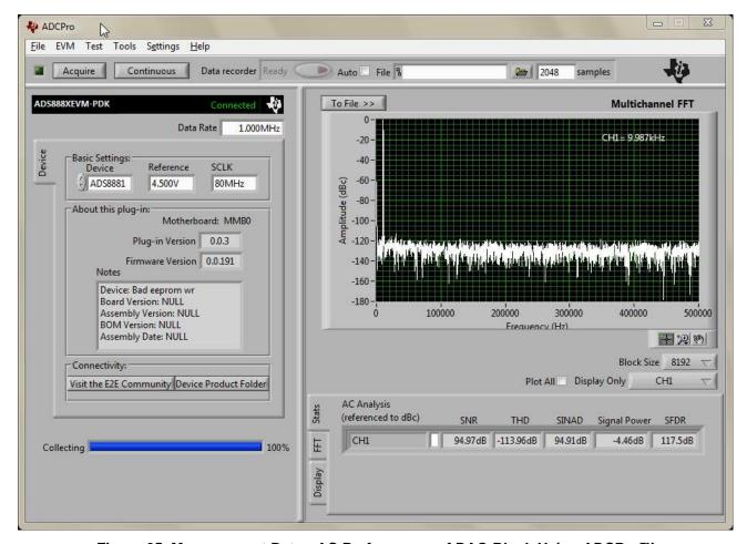
Figure 25. Measurement Data - AC Performance of DAQ Block Using ADCPro™
