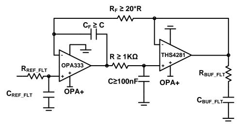
Figure 11. Schematic of Reference Buffer Circuit
