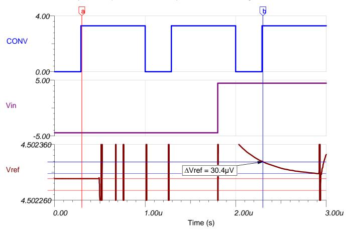
Figure 19. TINA-TI™ Simulation Result - ADC Reference Settling
