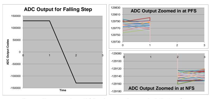
Figure 24. Measurement Data - ADC Transient Output Response for Falling Input Step
