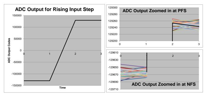
Figure 23. Measurement Data - ADC Transient Output Response for Rising Input Step
