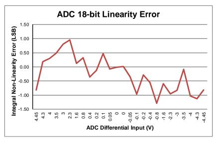
Figure 22. Measurement Data - ADC INL Plot (26-points)
