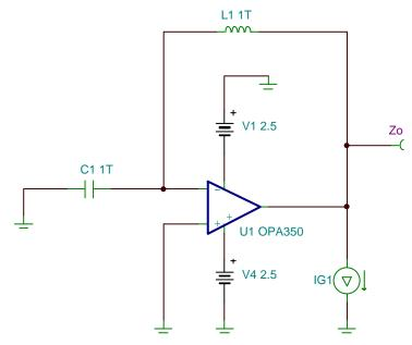
Figure 9. TINA-TI™ Schematic: Measuring Output Impedance of OPA350
