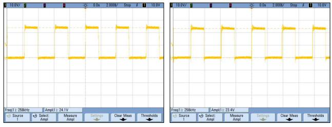
Figure 12. Switching Waveform at (Left) No Load at 24-V<sub>IN</sub> and (Right) Full Load at 24-V<sub>IN</sub>
