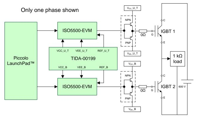
Figure 21. Setup for Testing TIDA-00199 Design With TI's ISO5500 and IGBTs
