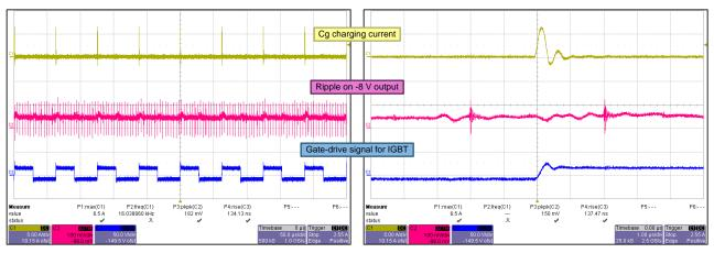
Figure 26. (A) Ripple on -8-V Output for 6-A Peak Load Current With IGBTs (B) Zoomed Waveforms
