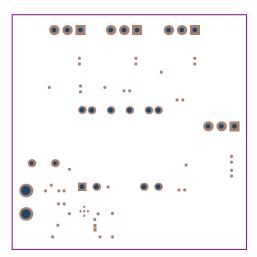
Figure 34. Bottom Solder Mask
