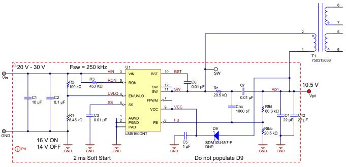
Figure 8. Primary Section of Schematic Showing LM5160
