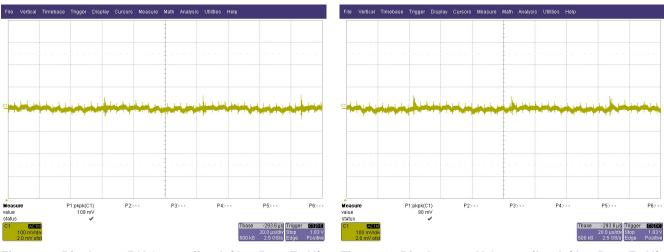
Figure 23. Ripple on 15-V Output (for dv/dt = 5.6 × E9 V/s on the Output Load)
