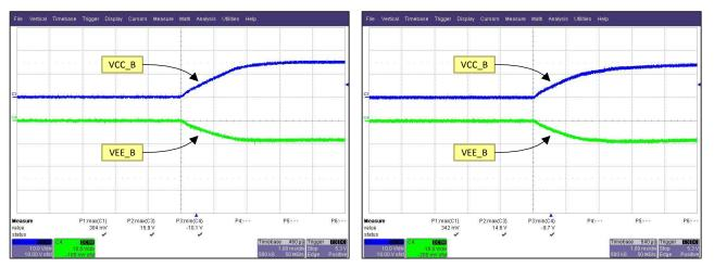
Figure 11. VCC\_B and VEE\_B Start-Up into (Left) No Load at 24-V<sub>IN</sub> and (Right) Full Load at 24-V<sub>IN</sub>
