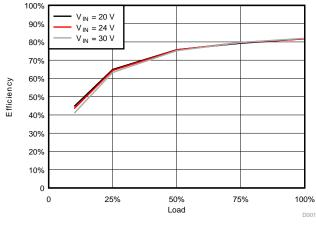
Figure 15. Total Efficiency Under Balanced Load
