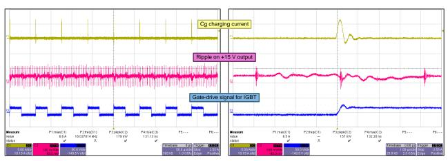
Figure 25. (A) Ripple on 15-V Output for 6-A Peak Load Current With IGBTs (B) Zoomed Waveforms
