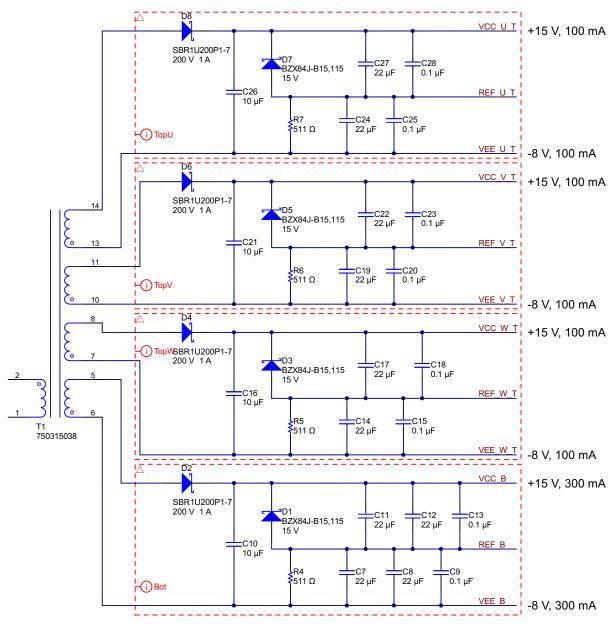
Figure 9. Secondary Section of the Schematic
