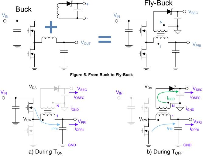
Figure 6. The Fly-Buck in ON and OFF time
