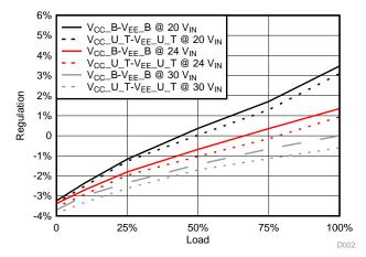
Figure 16.  $V_{cc}$  to  $V_{EE}$  Output Regulation Under Balanced Load
