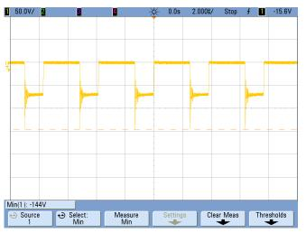
Figure 14. Bottom Output Diode Voltage at Full Load at  $30-V_{IN}$
