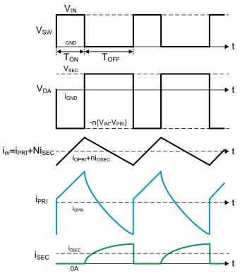
Figure 7. Fly-Buck Operation Waveform
