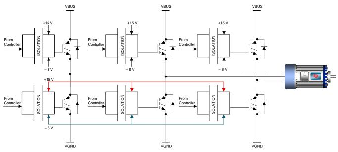
Figure 1. 3-Phase Inverter With Isolated Gate-drive
