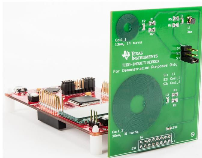
Figure 11. Sensor Board and LaunchPad Connection (Future Revisions After Rev. 1.0)
