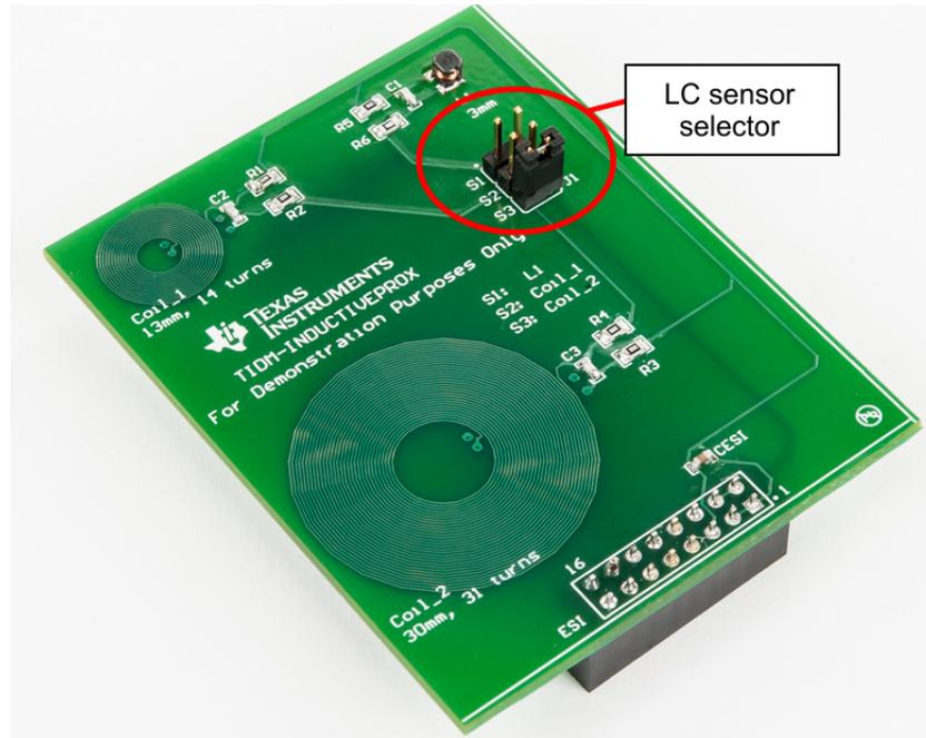
Figure 12. LC Sensor Selector
