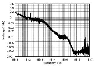
Figure 17. Output Noise—Two Parallel LDOs (Noise<sub>10 Hz</sub> - $_{100 \text{ kHz}} = 5.98 \ \mu V_{\text{RMS}}$
