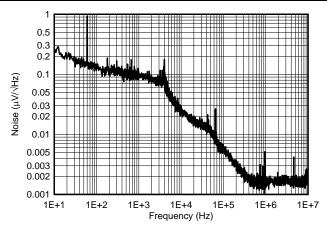
Figure 16. Output Noise—One LDO (Noise<sub>10 Hz - 100 kHz</sub> = 7.69 μV<sub>RMS</sub>)
