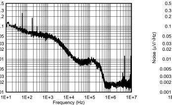
Figure 18. Output Noise—Four Parallel LDOs (Noise<sub>10 Hz</sub> - $_{100 \text{ kHz}} = 4.32 \ \mu V_{\text{RMS}}$
