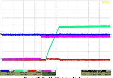
Figure 15. Enable Start-up—No Load
