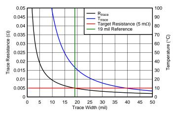
Figure 4. 400-mil Length PCB Trace Width versus Trace Resistance ( $\Omega$ )
