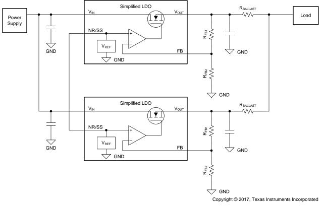
Figure 1. Two LDOs With Ballast Resistors
