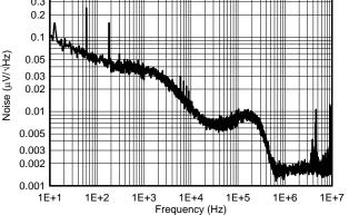
Figure 19. Output Noise—Eight Parallel LDOs (Noise 10 Hz - $_{100 \text{ kHz}} = 3.33 \, \mu \text{V}_{\text{RMS}}$
