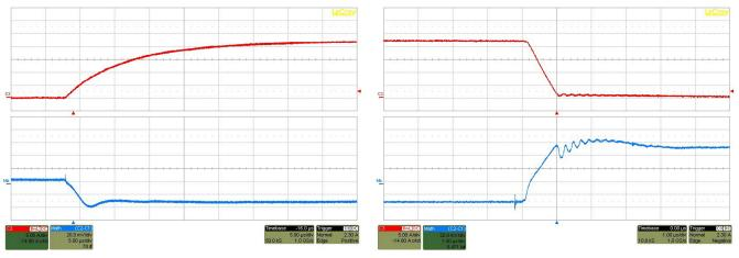
Figure 36. Load Transient 0 A to 23 A
