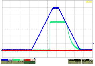
Figure 8. Start-up—Six LDOs, No Load
