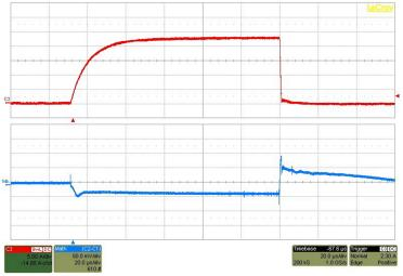
Figure 38. Load Transient 23 A
