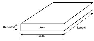
Figure 3. PCB Trace Dimensions
