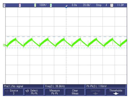
Figure 21. ISOW7841 DC Output Ripple
