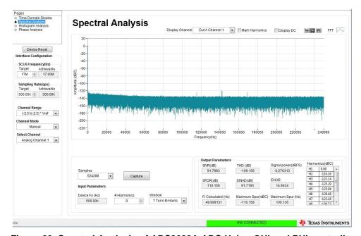
Figure 20. Spectral Analysis of ADS8688A ADC Using GUI and PHI controller
