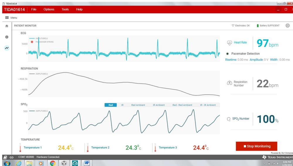
Figure 28. GUI Displaying ECG, Respiration and SPO2 Waveforms With SPO2 Number and Heart Rate
