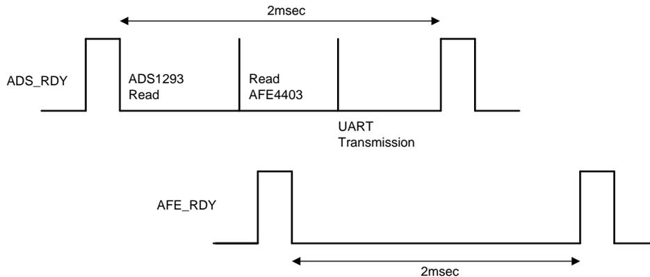
Figure 10 shows ADS1292R and AFE4403 Read and UART transmission (AFE4403 RDY comes while reading ADS1292).
