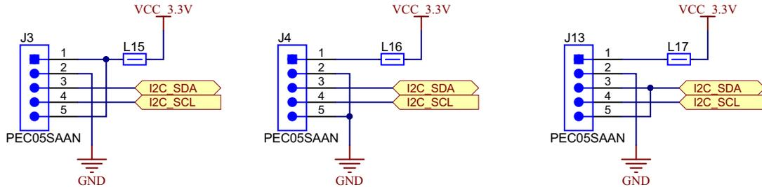
Figure 19 shows the connection to the temperature sensor TMP117. Three TMP117 temperature sensors are used for accurate measurement. Interface is from the I2C to the MCU. ADD0 pin is the fifth pin and connects to GND, V1, and SDA lines to select the unique slave address.
