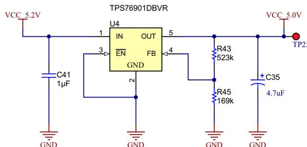
Figure 14 shows the LDO circuit generating 5 V from a 5.2-V input using the TPS76901. The 5 V provides the LED\_DRV\_SUP and TX\_CTRL\_SUP of the AFE4403 IC. The TPS76901 device is an ultra-low power 100-mA low-dropout linear regulator.
