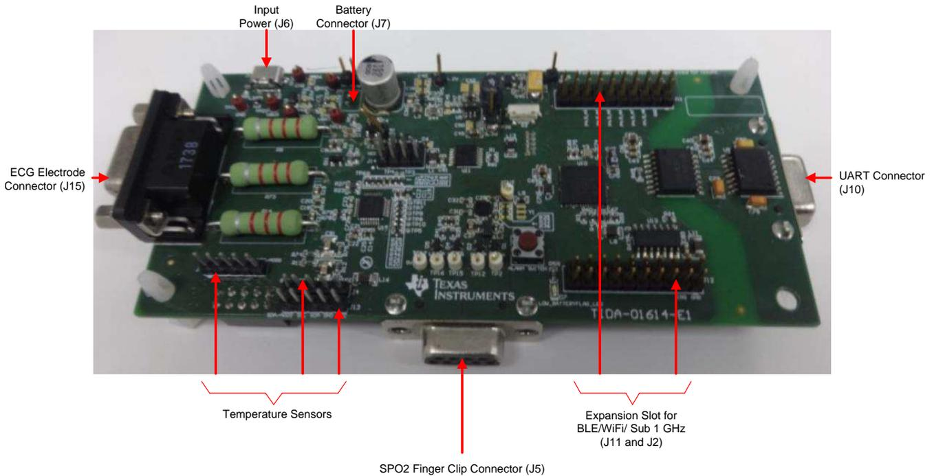
Figure 22. TIDA-01614 PCB Connector Configuration – Bottom View
