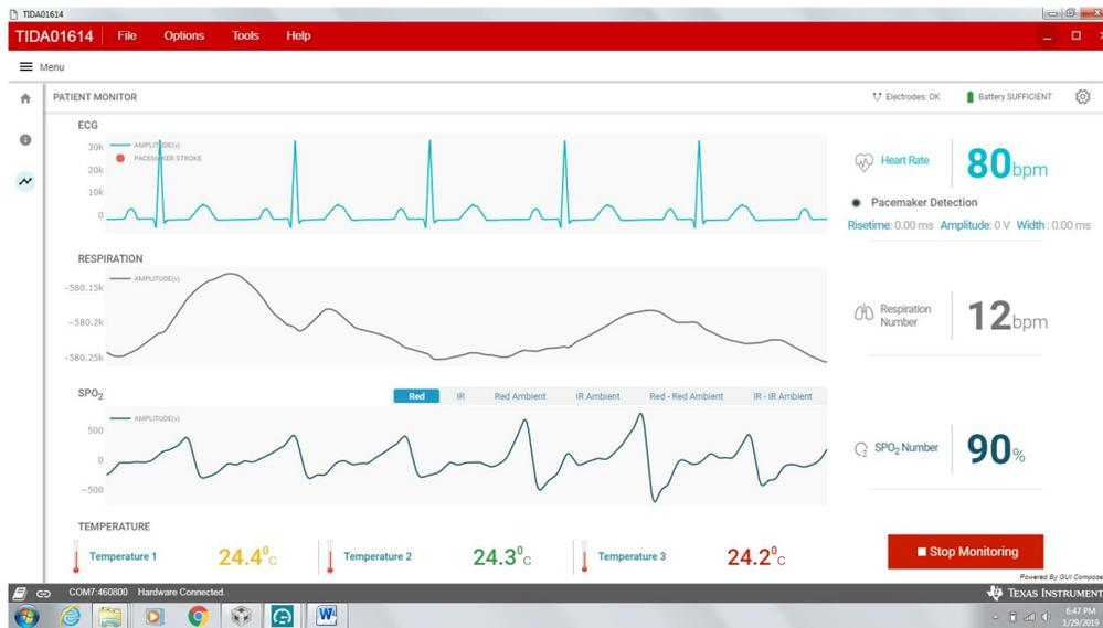
Figure 27. GUI Displaying ECG, SPO2 Waveforms With SPO2 Number and Heart Rate With ECG Sensitivity of 100- $\mu$ Vs
