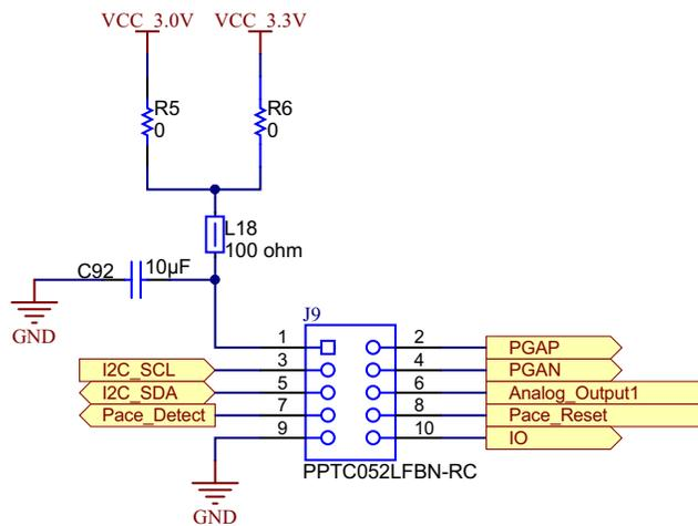
J9 represents the connection to the pace detection module (TIDA-010005). The pace detection module is interfaced from the I2C to the main TIDA board. PGAP and PGAN from ADS1292R IC of the TIDA-01614 board goes to the pace detection module and detects if any pace pulse is present in the ECG waveform and gives a pace detect to the MCU. Pace reset resets all the counters on the TIDA-010005 board.
